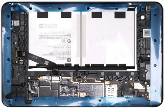
Then stick on the new screen back glue.
