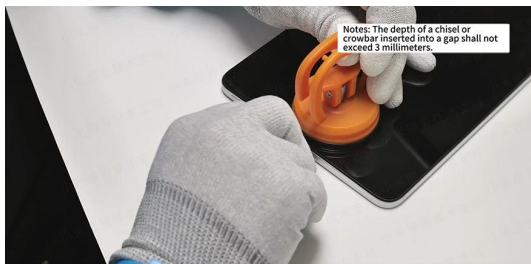
Insert the disassembly slider from the touch screen
