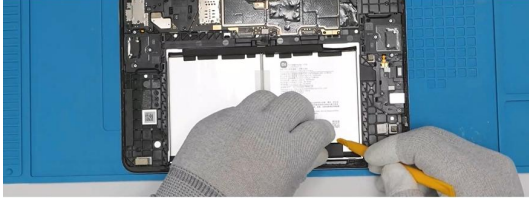
Use a pry bar and hands to gently tear off the black film.
