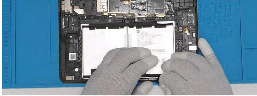
After tearing off the black film, don't pull it directly.
