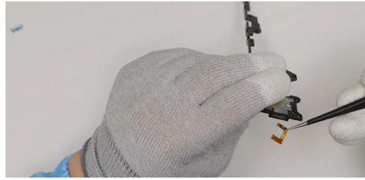
FPC from the bracket assembly limit position.
