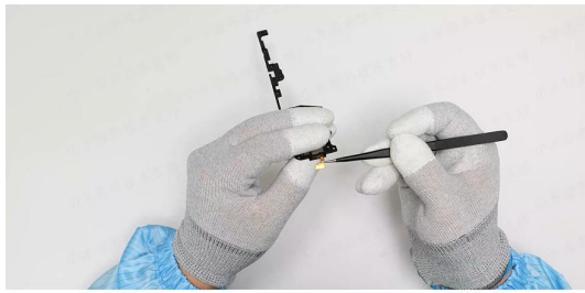
Install the power button FPC to the front camera
