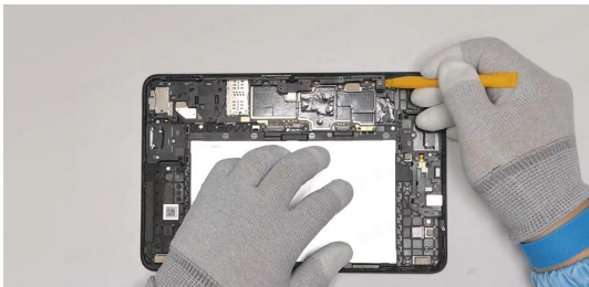
Gently lift and remove the front and rear camera brackets.
