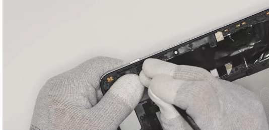
Use the tweezers to press the volume and power buttons inward.
