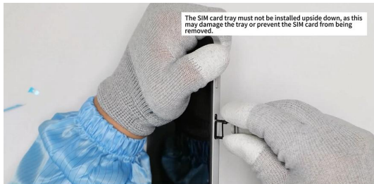
Insert the SIM card tray directly into the phone's SIM card tray.
