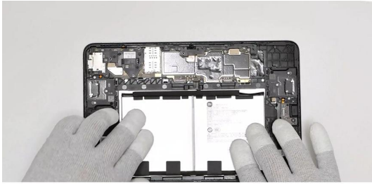
Make sure the battery is assembled flat and in place.
