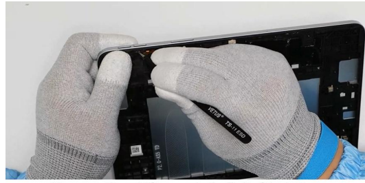
Then snap the gold finger onto the limit of the battery cover.
