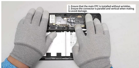
Connect the main FPC main board connector to the main board.
