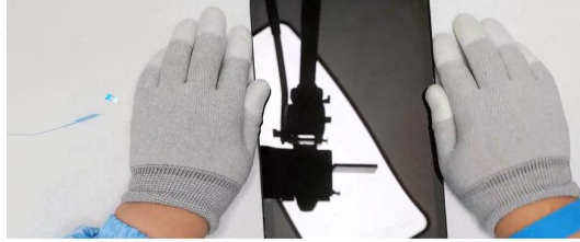
Put it into the pressing jig and press it.
