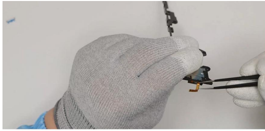
Then remove the power button's gold finger
