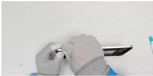
Finally, install the volume key to
