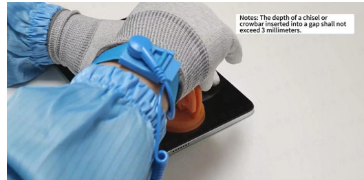
After sucking up the gap with a suction cup,
