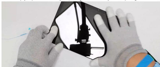
Press the entire touch display assembly
