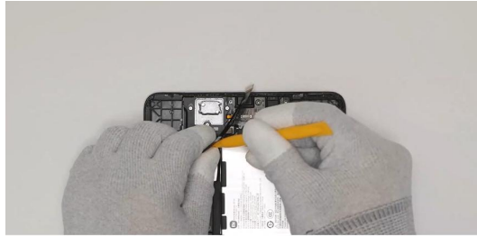
the sub-board connector and remove it.
