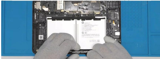
Pull the white glue out at a constant speed.
