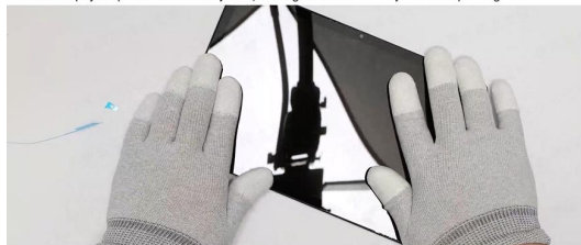
and press the four sides of the touch display component.
