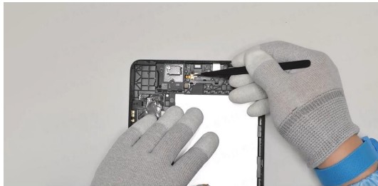
Insert the tweezers into the FPC gold finger of the speaker
