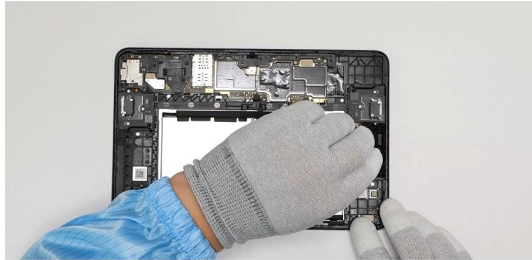
Fasten the compression bracket to the sub-board.
