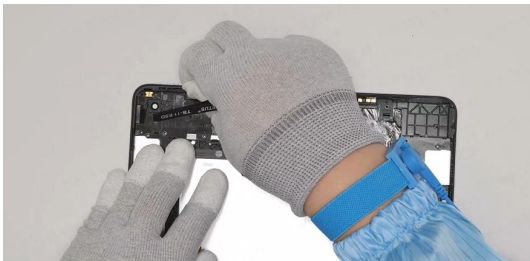
Finally, use tweezers to pick up the volume key FPC assembly.
