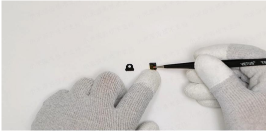
Remove the front camera's protective film.
