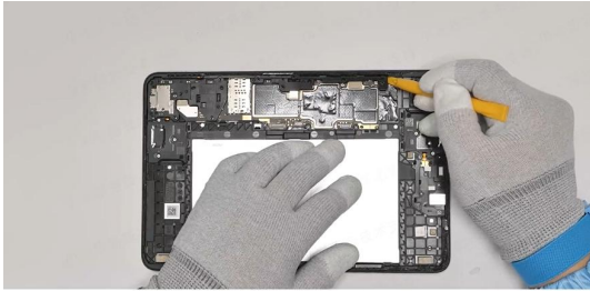
Use the disassembly stick at the corresponding position
