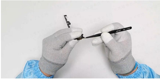
Stick a new power key waterproof foam.
