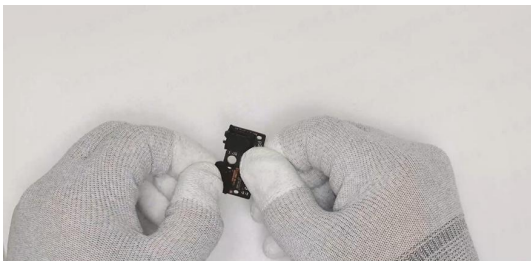
and gently separate the USB rubber sleeve
