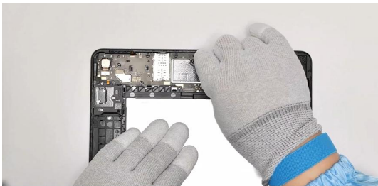
Connect the front camera connector
