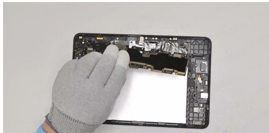
to lift and remove the motherboard.
