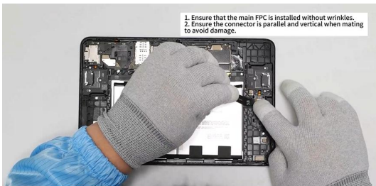
Connect the main FPC connector to the sub-board connector.
