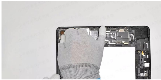
Connect the rear camera connector
