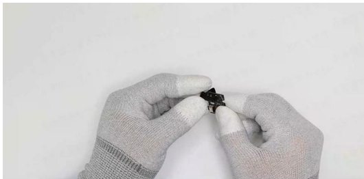
Install the earphone jack rubber sleeve and USB rubber sleeve
