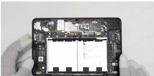
Make sure the battery and battery cover are firmly attached.
