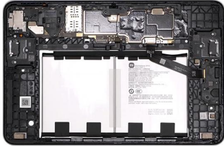
Use a screwdriver to install the motherboard
