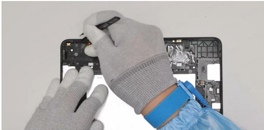
Use tweezers to gently tear off the waterproof foam.
