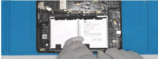
Feel no obstruction and pull out a section of white glue.
