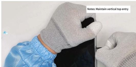
Then remove the SIM card tray.
