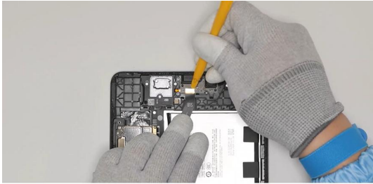
Use a disassembly stick to gently lift and remove
