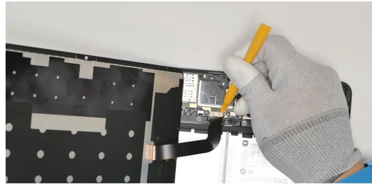
the screen FPC connector interface on the main board
