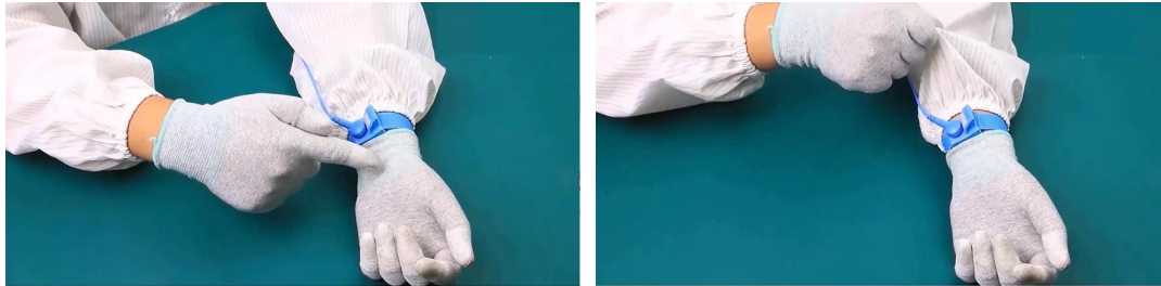
Before the disassembly and assembly, ensure that you are wearing anti-static gloves, wristbands and clothing
