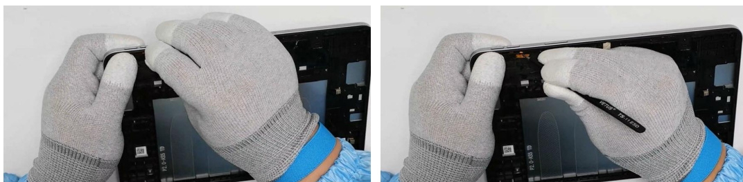
Install the volume key FPC to
