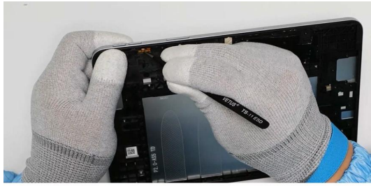
Stick the new volume key waterproof foam.
