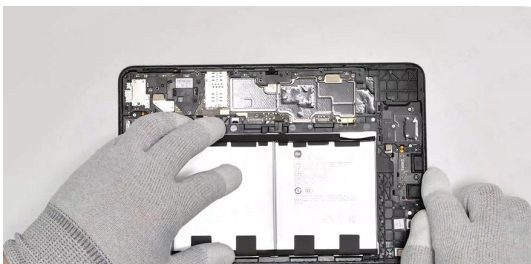
Activate the easy-release tape.
