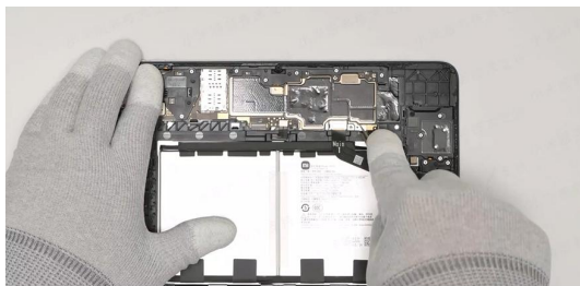
Use tweezers to gently pick up and remove the holder.
