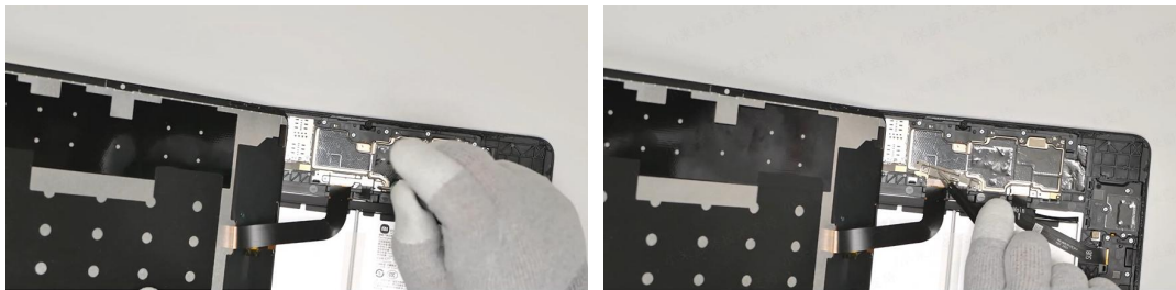
Use a screwdriver to remove two screws.
