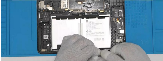
Hold the black film and shake it left and right.
