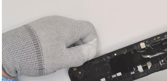
Use the tweezers to press the volume and power buttons inward.
