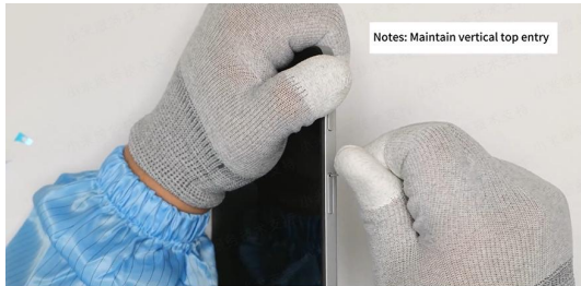
Push the opening pin into the body with force
