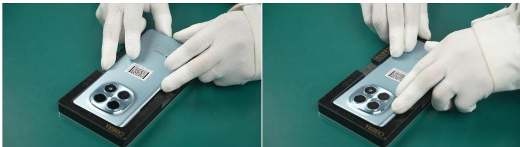
(3) Tear off the protective film on the other side of the Battery Cover Adhesive, align the Battery Cover Assy with the device, and press gently to install it in place.
