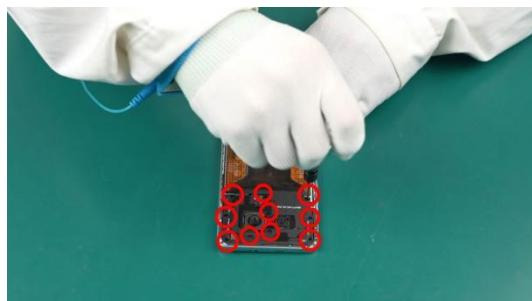
i Check the number of screws that have been removed and keep them in a safe place to ensure that no unassembled screws are left inside the device during the assembly process.
