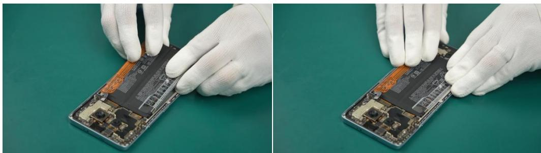
(3) Finally connect the Battery to the Mainboard Assy.
