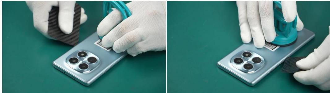
💡 Use the Plastic Pry Tool to slide along the left edge of the device to cut the glue, leaving the Plastic Pry Tool on the left edge side when finished to prevent the adhesive from resealing.
