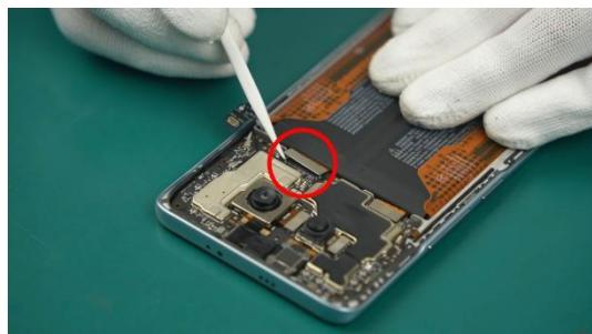
(3) Disconnect the FPC Assy-Mainboard\_subboard from the Mainboard Assy.
