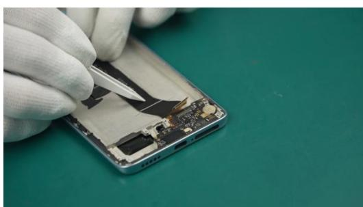
i Be careful not to damage the cable when arranging it.
