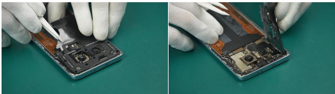
i Pay attention to the clips around the Mainboard Cover Assy during operation. Make sure the clips are completely separated before proceeding to the next step to avoid damaging the Mainboard Cover Assy.
