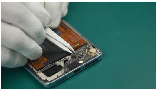
i Pay attention to the clips around the Sub-Board Assy during operation. Make sure the clips are completely separated before proceeding to the next step to avoid damaging the Sub-Board Assy.
