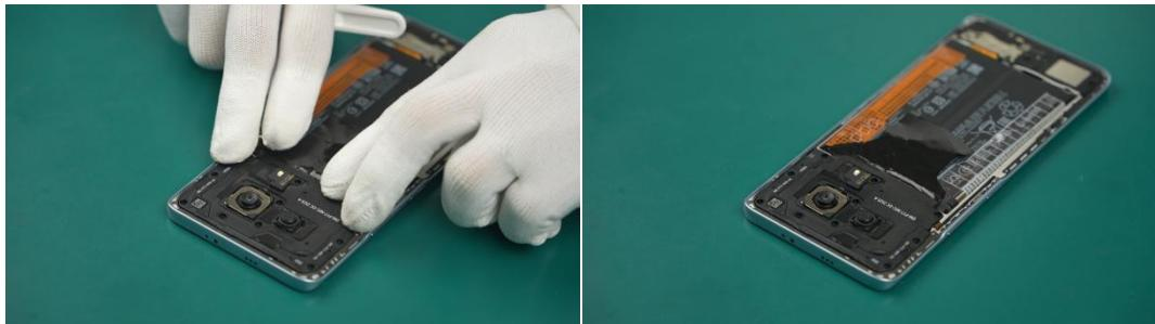
(2) Align the screw holes and tighten the screws.
