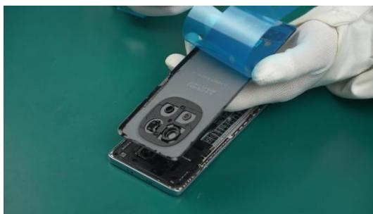
(4) Align the Battery Cover Assy with the device, and press gently to install it in place.
