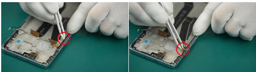
i During the subsequent assembly process, you need to check whether the Side Key FPC harness is lifted up to avoid squeezing the harness during assembly.
