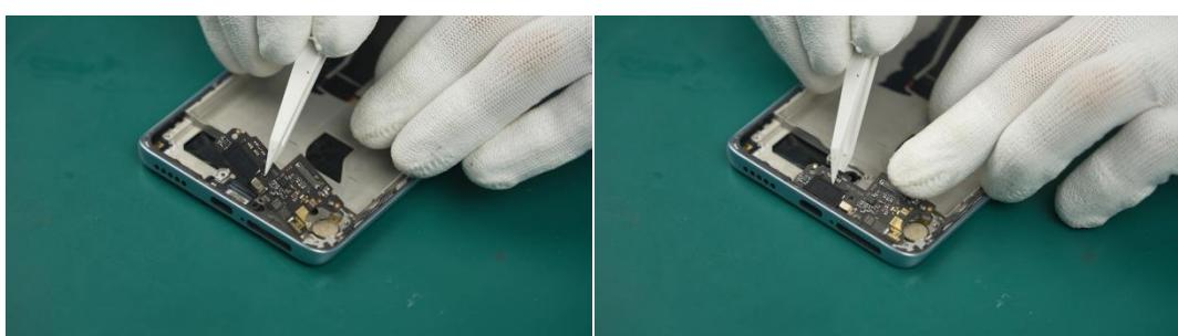
i Please check the components underneath when installing the Sub-Board Assy. If the components underneath are not properly installed, the Sub-Board Assy may not be properly installed.
