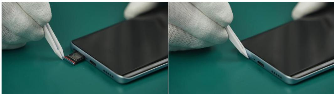
i Please do not use hard tools to install the SIM card tray to avoid scratching the device.
