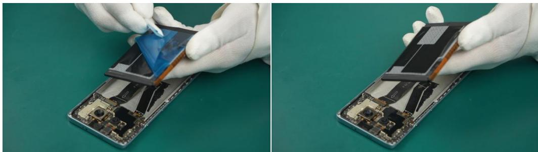
(2) Align the phone to the correct position, put the Battery in, and press lightly to ensure a firm fit.
