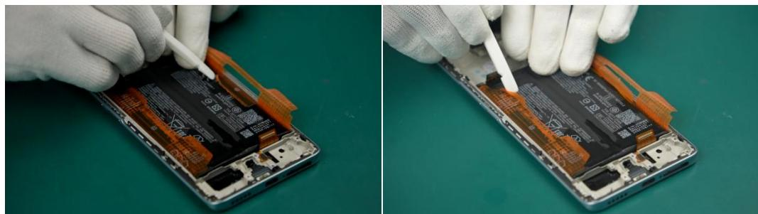
(2) Remove the Battery and tear off the remaining Easy release adhesive on the device.
