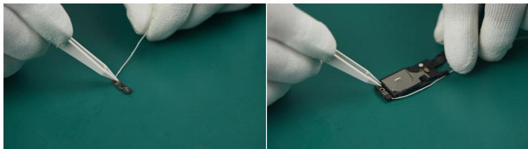
i Be careful not to damage the cable when arranging it.
