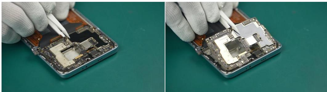
i Carefully lift the Mainboard Assy with tweezers and remove the Mainboard Assy, being careful not to damage the PBA board.
