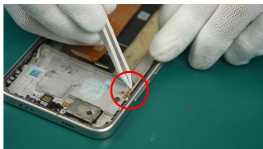
i During the subsequent assembly process, you need to check whether the Holder-Side Key FPC harness is lifted up to avoid squeezing the harness during assembly.
