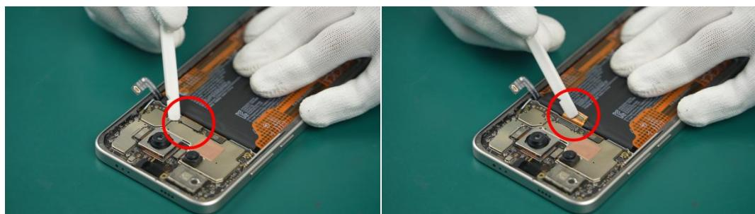
(3) Disconnect the FPC Assy-TP Transfer from the Mainboard Assy.
