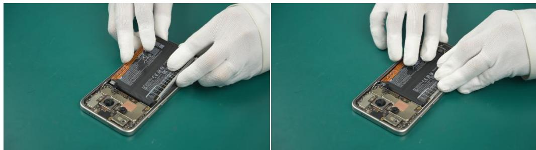
(3) Connect the Battery to the Mainboard Assy.
