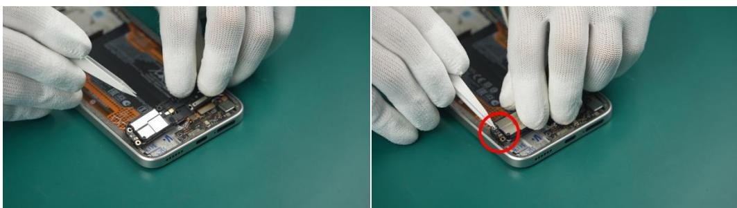
i Do not use metal tools during operation to avoid scratching the device.
