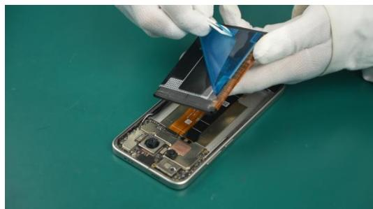
(2) Align the phone to the correct position, put the Battery in, and press lightly to ensure a firm fit.
