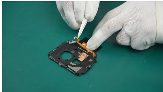
i Pay attention to the clips around the Mainboard cover Assy during operation. Make sure the clips are completely separated before proceeding to the next step to avoid damaging the Mainboard cover Assy.
