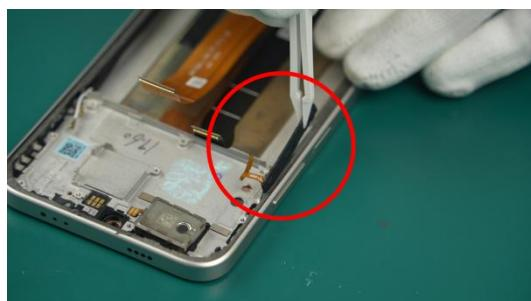
(2) Place the Side Key FPC into the correct position, press to ensure it clicks into place.
