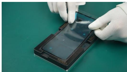
(2) Tear off the protective film of the Battery Cover Adhesive, and do not touch the adhesive surface.
