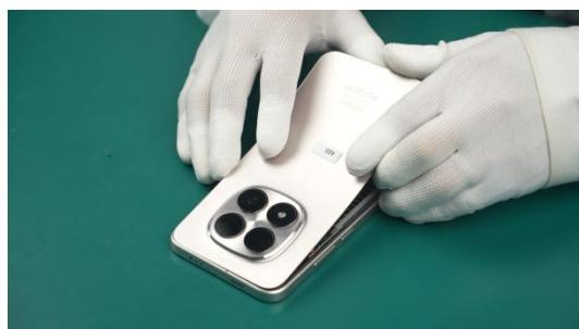
! Place the phone into the Battery cover assembly press device and crimp it for 60 seconds using the Crimping tool.
