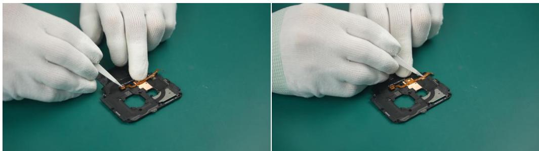
i Please ensure that the Main FPC Assy fits flatly with the device to avoid damage to the Main FPC Assy caused by squeezing other accessories during subsequent assembly.
