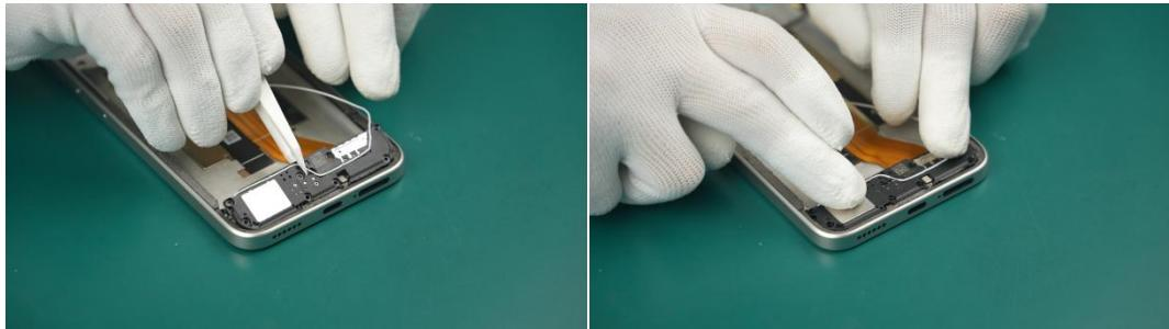
(2) Flip the Sub-Board cover and press the Coaxial Cable-White into the wire groove of the Sub-Board cover.
