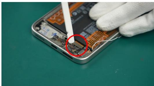
i Do not use metal tools during operation to avoid scratching the device.
