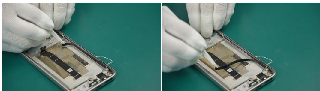
(2) Remove the Coaxial Cable-White and Coaxial Cable-Black from the device.
