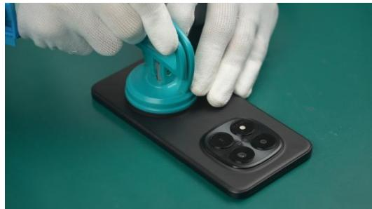
(2) Use a plastic pry tool to slowly separate the Battery Cover Assy from the device.
