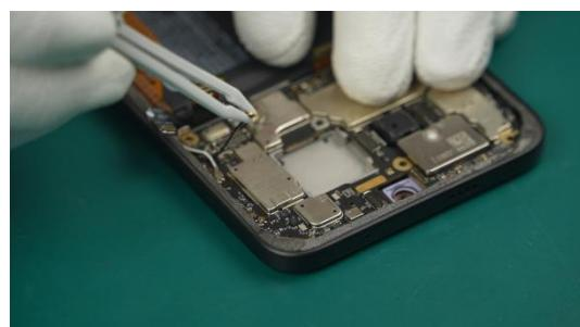
i Do not pull the cable directly when disconnecting to avoid breaking it.
