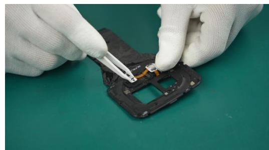
(2) Connect the FPC Assy-Flash Light to the Mainboard Assy.
