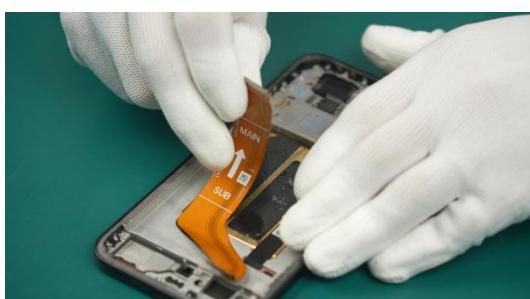
💡 You can use special alcohol to help remove the adhesive, or use the microwave to heat the heating bags, then heat the device before removing it.
