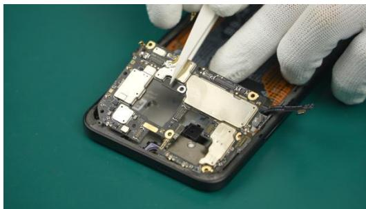
i Carefully lift the Mainboard Assy with tweezers and remove the Mainboard Assy, being careful not to damage the PBA board.
