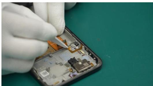
i During the subsequent installation process, you need to check whether the Side Key FPC harness is lifted up to avoid squeezing the harness during installation.
