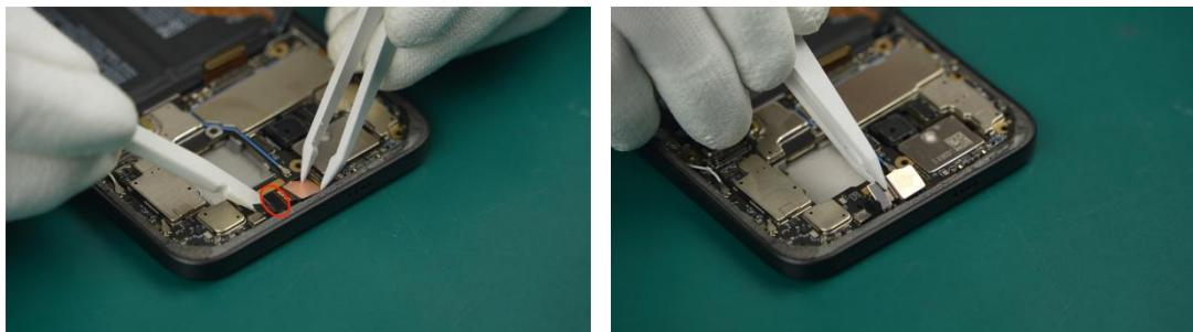
i Do not touch the camera lens directly during operation to avoid scratching the lens.
