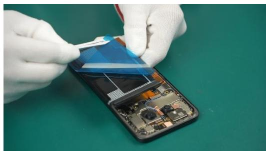
(2) Align it with the correct position on the phone, insert the Battery, and press gently to ensure a secure fit.
