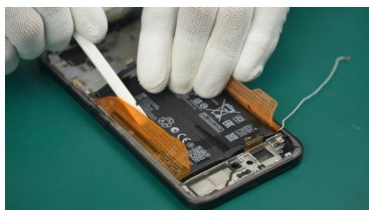
(2) Remove the Battery and tear off the remaining Easy Release Adhesive on the device.
