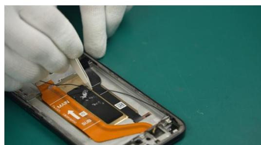
i Do not pull the interface of the Coaxial Cable to avoid breaking the interface of the Coaxial Cable.
