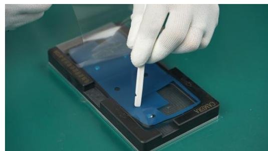
(2) Put the Battery Cover Assy into the Adhesive backing fixing tool, press gently to make the Battery Cover Assy Adhesive and the Battery Cover Assy fit together.
