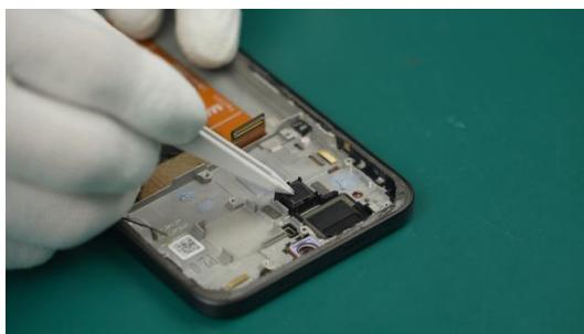
(2) Place the Top Speaker Assy into the correct position on the device, and gently press it to make sure it is securely in place.
