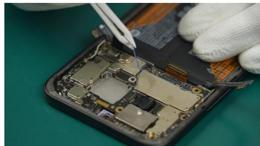
i Be careful not to damage the wiring harness interface and surrounding components during operation.
