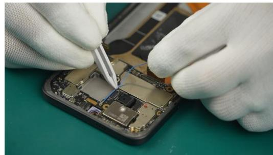
(2) Connect the other end of Coaxial Cable-Blue to the Mainboard Assy.
