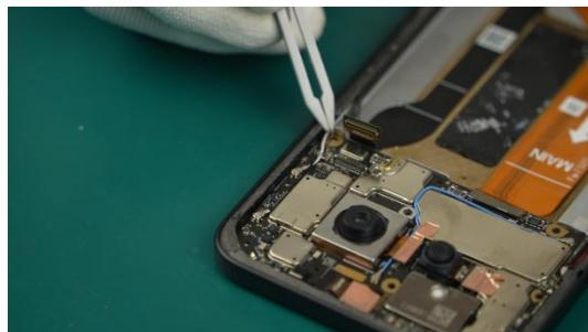
⚠ Be careful not to damage the wiring harness when arranging it.
