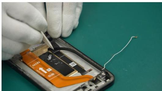
(2) Remove the Coaxial Cable-White and Coaxial Cable-Black from the device.
