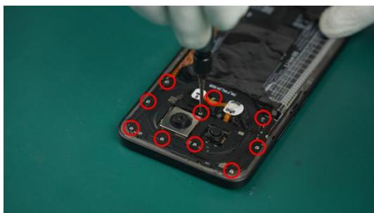
i Please check the number of screws installed to ensure that no unassembled screws are left inside the device.
