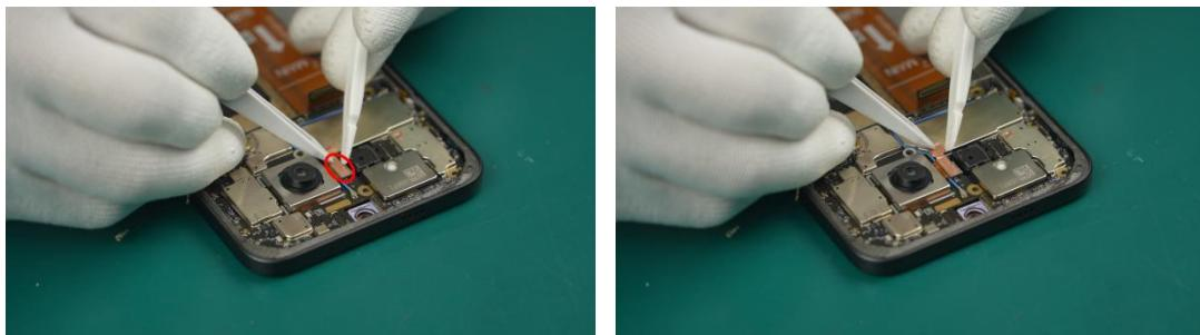
(4) Connect the Camera-Rear-Ultra Wide Angle to the Mainboard Assy and ensure the copper foil is properly attached.
