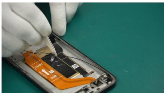
i Do not pull the interface of the Coaxial Cable to avoid breaking the interface of the Coaxial Cable.
