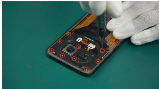
i Check the number of screws that have been removed and keep them in a safe place to ensure that no unassembled screws are left inside the device during the assembly process.
