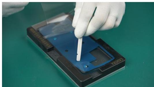
(2) Put the Battery Cover Assy into the Adhesive backing fixing tool, press gently to make the Battery Cover Assy Adhesive and the Battery Cover Assy fit together.
