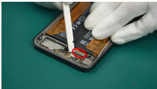
i Please disconnect the interface in parallel during operation to avoid tilting and pulling, which may cause damage to the interface.
