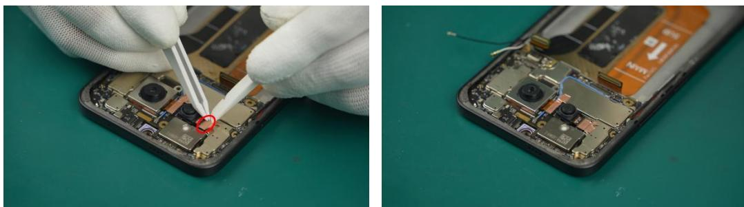
(5) Connect the Camera-Front to the Mainboard Assy, and ensure the copper foil of the Camera-Front is properly attached.
