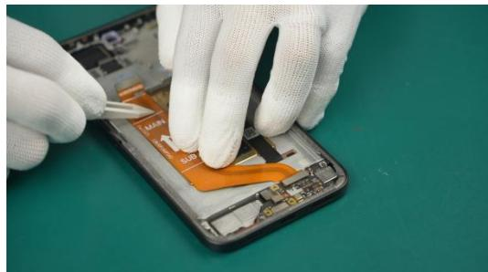
i During the subsequent assembly process, you need to check whether the FPC Assy is lifted up to avoid squeezing the cable during assembly.
