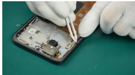
(2) Tidy up the cable to ensure it is installed in place.
