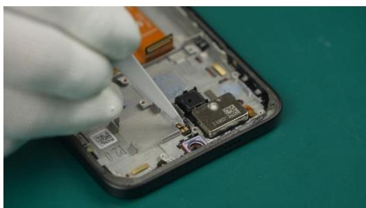
i Do not use metal tools to press to avoid damaging the Light Sensor Board Assy.
