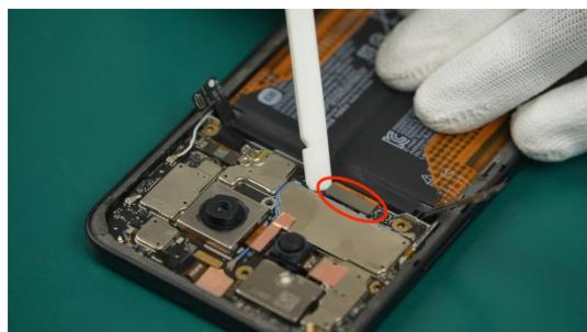
(4) Disconnect the Front Cover Display Module from the Mainboard Assy.
