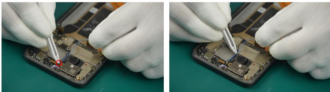
(2) Connect the other end of Coaxial Cable-Blue to the Mainboard Assy.
