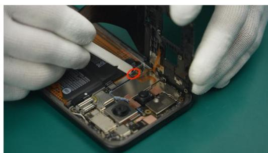
i Pay attention to the clips around the Flash Lampshade during operation. Make sure the clips are completely separated before proceeding to the next step to avoid damaging the Flash Lampshade.
