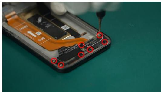
i Check the number of screws installed to ensure that no unassembled screws were left inside the device during assembly.
