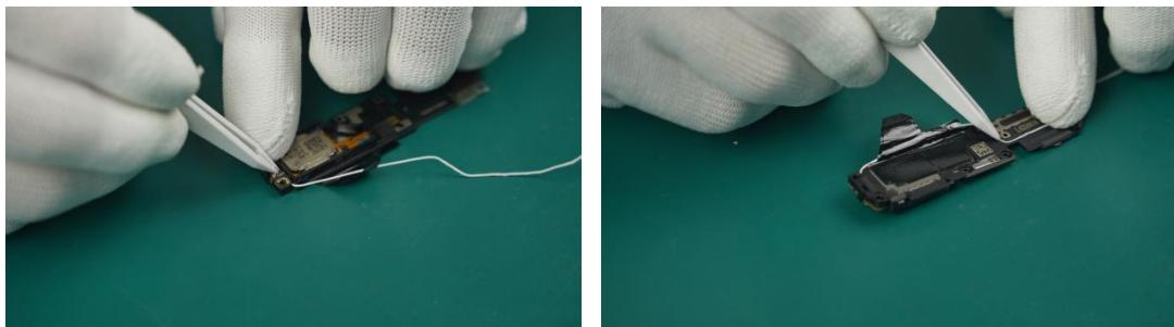
i Be careful not to damage the wiring harness when arranging it.
