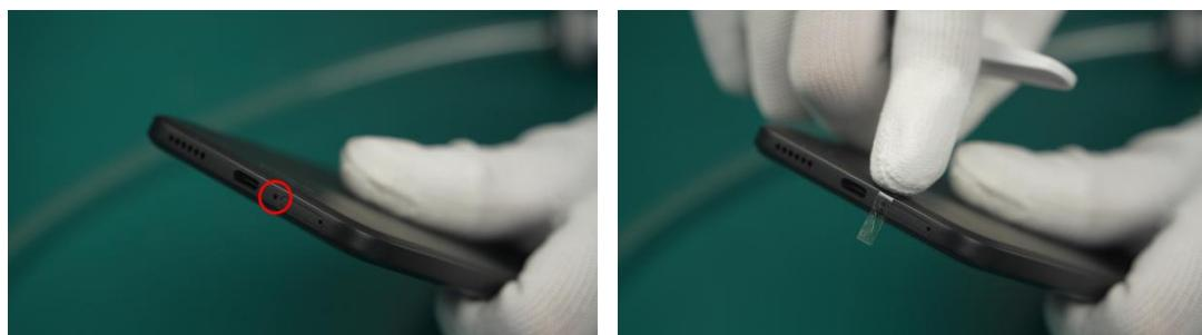
(3) Use the Air tightness tester, aim at the air tightness test hole(The outermost hole of the speaker), and perform the test. If "OK" is displayed on the screen, it means that the mobile phone has passed the test.
