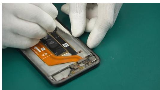
(2) Connect the Coaxial Cable-White to the Antenna Board Assy.
