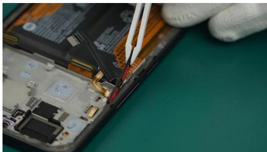
💡 Use ESD Safe Tweezers to cut the adhesive between the Holder-Side Key FPC and the device. Use ESD Safe Tweezers to press one side of the Holder-Side Key FPC in the slot to lift up the other side of the Holder-Side Key FPC. Then use ESD Safe Tweezers to remove the Holder-Side Key FPC.
