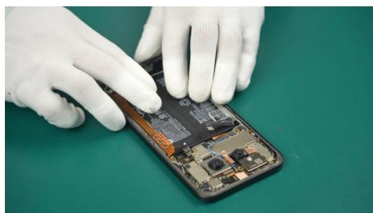
i Please try not to touch the surface of the Easy Release Adhesive to avoid contamination of the Easy Release Adhesive and affecting the adhesion effect.
