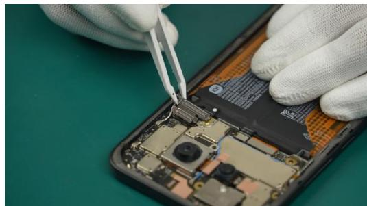
i Please keep small parts properly, as missing parts may cause the device to fail to start up.
