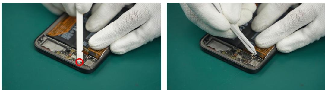
i Please disconnect the interface in parallel during operation to avoid tilting and pulling, which may cause damage to the interface.
