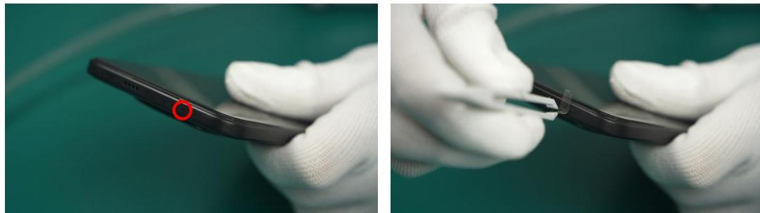
(2) Block the mic holes at the bottom of the phone.
