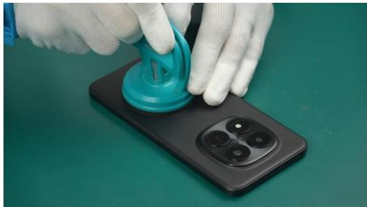
(2) Use a plastic pry tool to slowly separate the Battery Cover Assy from the device.
