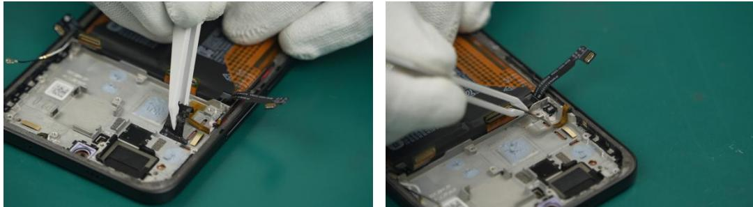
💡 You can use special alcohol to help tear off the PET Film-Isolating Cable.
