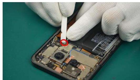
(4) Install the BTB steel sheet into place.
