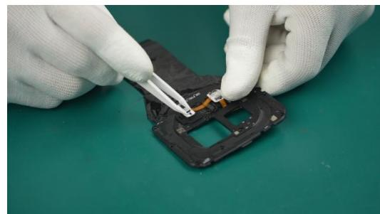
(2) Connect the FPC Assy-Flash Light to the Mainboard Assy.
