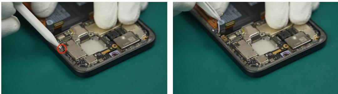
i Do not pull the cable directly when disconnecting to avoid breaking it.
