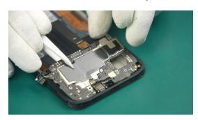
Carefully lift the Mainboard Assy with tweezers and remove the Mainboard Assy, being careful not to damage the PBA board.
