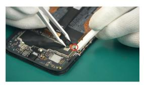
(3) Disconnect Camera-Front and remove it from the device.
