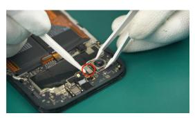
(2) Disconnect Camera-Rear-Macro-Depth and remove it from the device.
