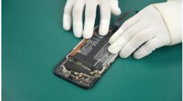
(3) Connect the Front Cover Display Module and the Battery to the Mainboard Assy.
