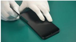
(3) Lift the Middle Frame Assy. Disconnect the cable of the Fingerprint Module from the device, and then remove the Middle Frame Assy;
