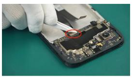
(2) Connect the Coaxial Cable to the Mainboard Assy.
