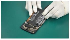
(5) Connect the Front Cover Display Module and the Battery to the Mainboard Assy.
