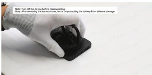
Use a suction cup to lift the gap.
