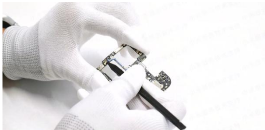
Remove the blue coaxial cable on the mainboard.
