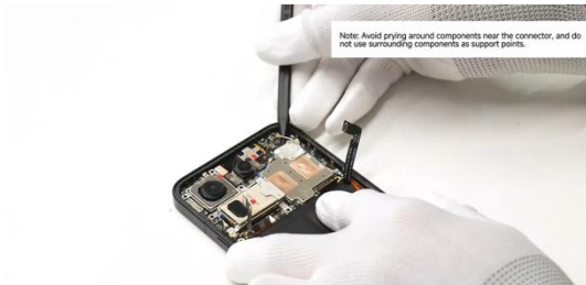
Disconnect the main FPC connector and the black and white coaxial cables.
