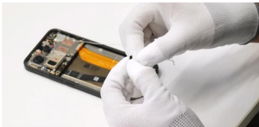
Connect the coaxial cable to the antenna board.
