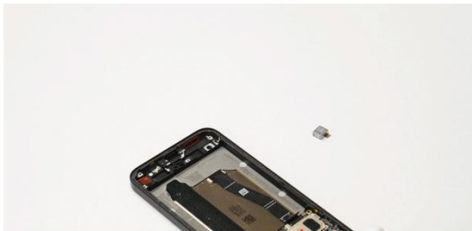
Apply motor adhesive.
