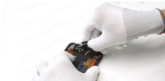
Use tweezers to lift the motor
