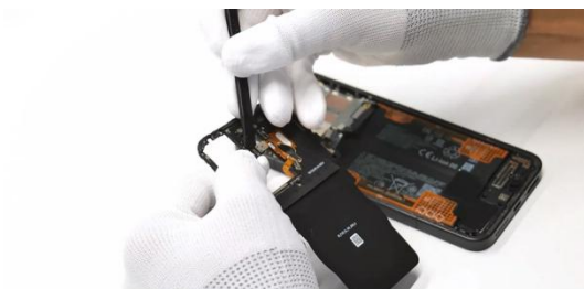
Disassemble the flash FPC component on the antenna back shell.
