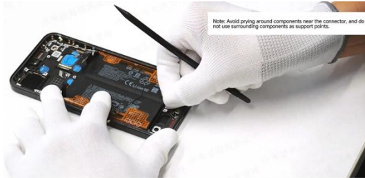
Disconnect the fingerprint connector, main FPC
