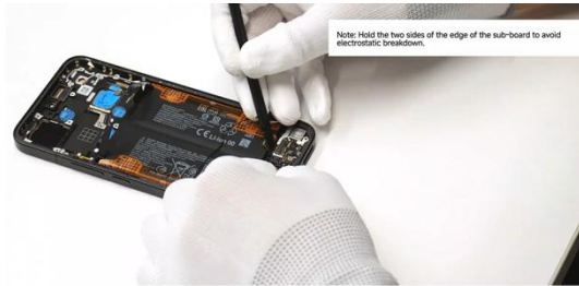
Use a pry bar to gently lift and remove
