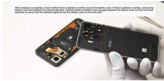
align one end of the battery cover with the front case.
