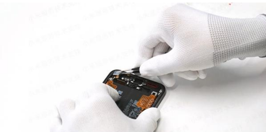
lift the motor from the removal position and remove it.
