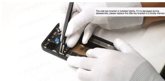
Gently lift the gold fingers of the side key FPC from the removal position.
