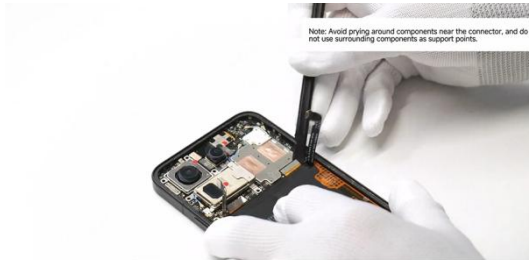
Disconnect the display FPC connector.
