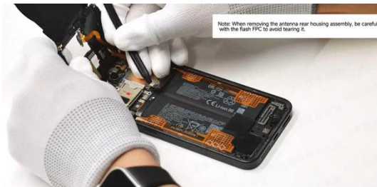
Disconnect battery connector one and two first.
