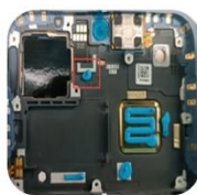
First, use a dispensing gun to apply thermal grease to the frame.
