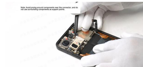
Use a pry bar to disconnect the periscope camera,
