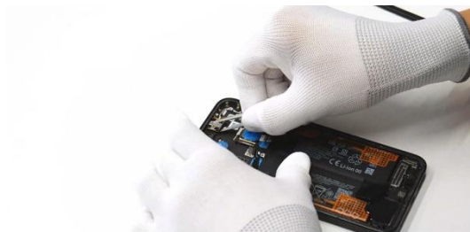
lift the FPC of the receiver from the gold finger.
