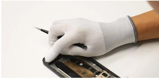
Press gently to activate the adhesive.
