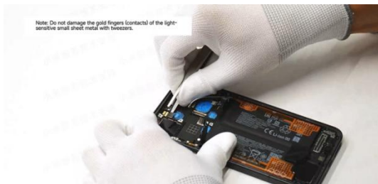
Use tweezers to gently lift the light sensor board.
