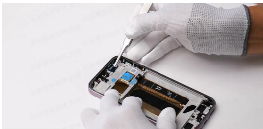
Apply the back glue to the receiver.
