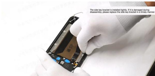
Use tweezers to lift the side key bracket from
