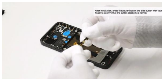
Insert the side key FPC assembly into the key slot.
