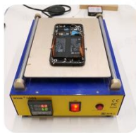
Heat the phone screen facing down.
