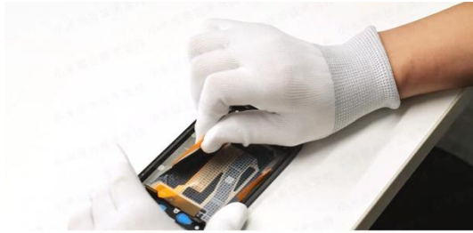
The battery cannot be reused after disassembly.
