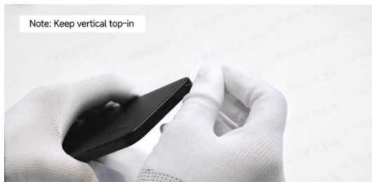
Push the opening pin into the phone with force
