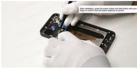
into the corresponding position of the middle frame.
