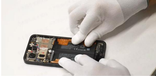
Assemble the battery into the battery compartment.
