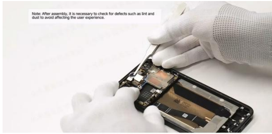
ensuring the interface is fastened smoothly.
