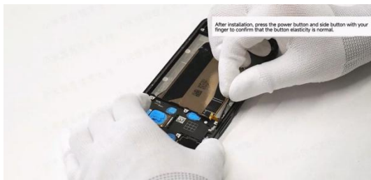
and then insert it into the side key position on the frame.
