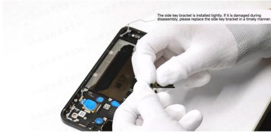
Separate the side key FPC from the side key bracket.
