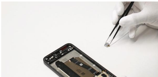
Use tweezers to pick up the vibrator.
