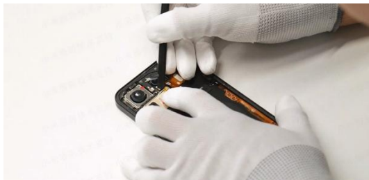
and stick the flash FPC to the periscope camera.
