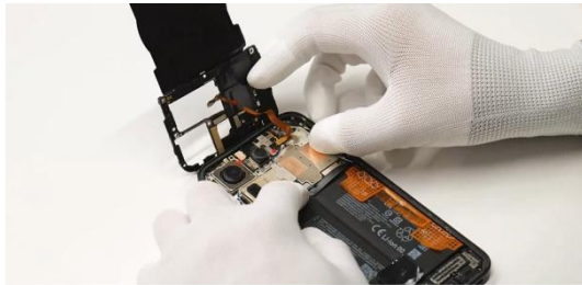
Fasten the battery connector.
