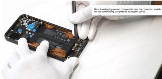
Disconnect the fingerprint connector, main FPC
