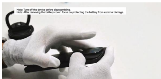
Completely separate the battery cover.
