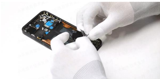
Separate the antenna board from the lower speaker.
