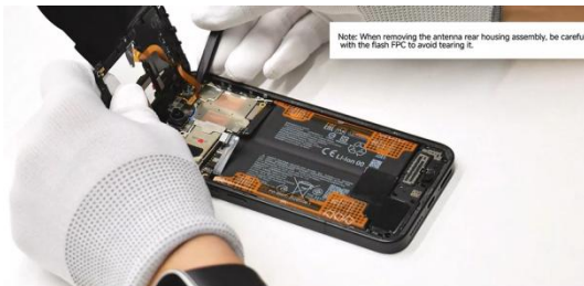
Disconnect the flash FPC BTB interface.
