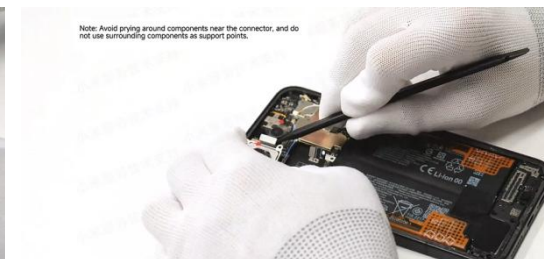
and remove the rear main camera, wide-angle camera connector.
