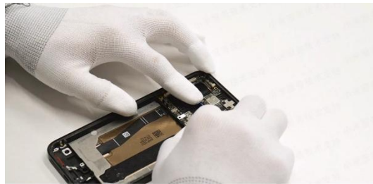
Then assemble it vertically downward to the frame.
