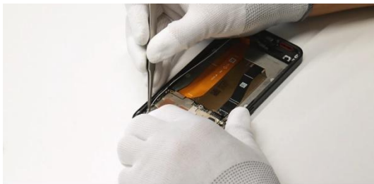
Assemble the white coaxial cable to the main and sub-board ends.
