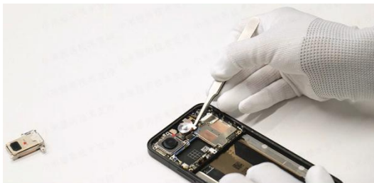
and periscope camera to the corresponding position.
