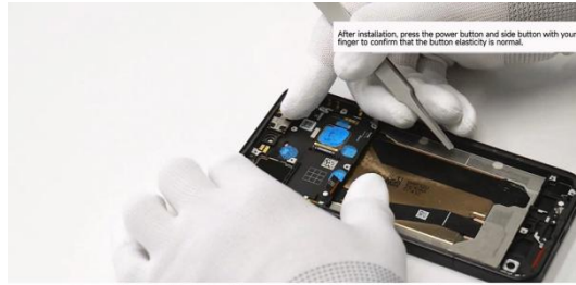
Organize and paste the receiver FPC into the frame limit slot.
