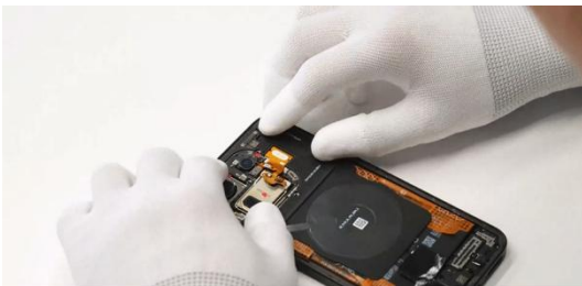
Align the antenna back shell assembly along
