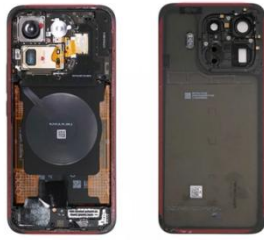
After disassembling, clean the residual glue on the battery cover
