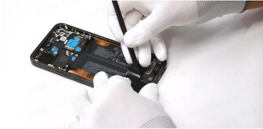
Use your hand or a pry bar to disassemble from the top.
