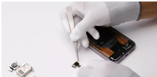
Protect the front camera with a protective film.
