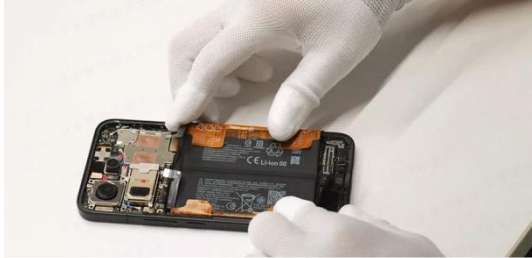
Peel off the release paper of the battery.
