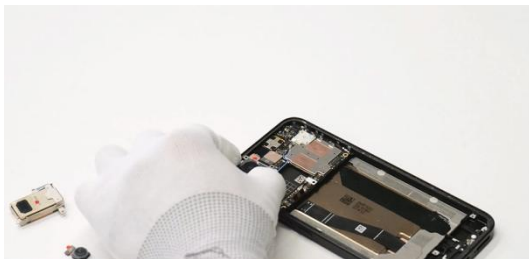
Install the rear main camera, wide-angle camera,
