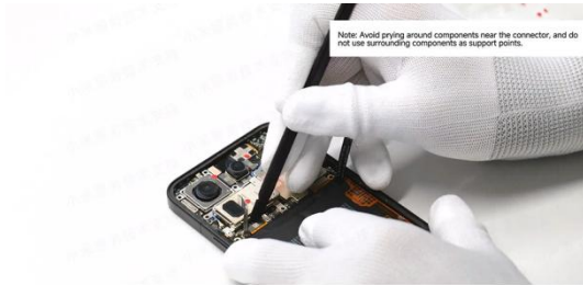
Use an anti-static plastic tweezers or a pry bar.
