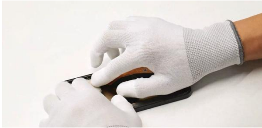
Align the main FPC in place.
