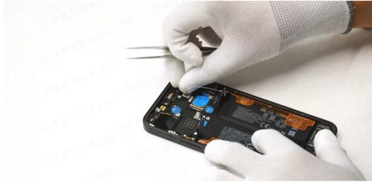
Clear the double-sided tape of the receiver seal.
