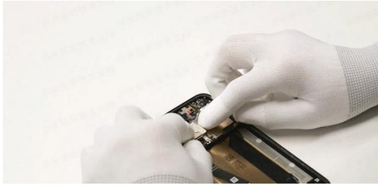
Make sure the interface is fastened in place.
