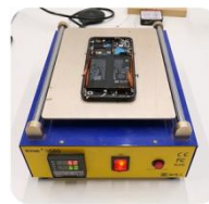
The heating temperature is sixty degrees Celsius.
