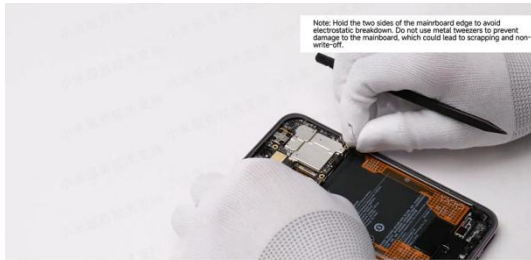
Remove the mainboard from the main camera notch.
