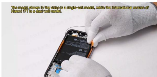
Use a suction cup or lift the battery handle
