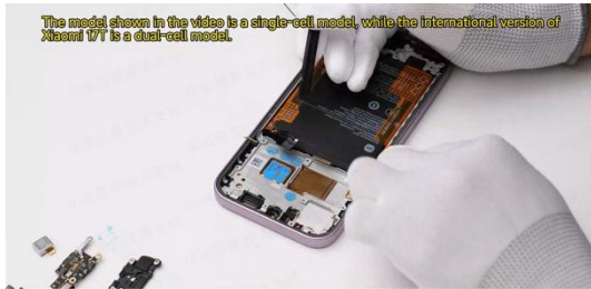
Peel off the battery's easy-tear glue.
