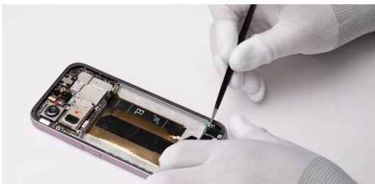
Apply motor adhesive.
