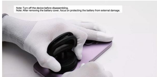
insert it into the body from the bottom side gap.
