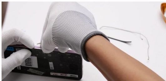
Use tweezers to push out the power and volume keys.
