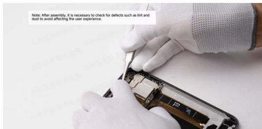
Apply graphite copper foil to the front camera.
