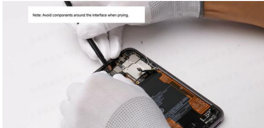
Use a disassembly stick to separate the front camera
