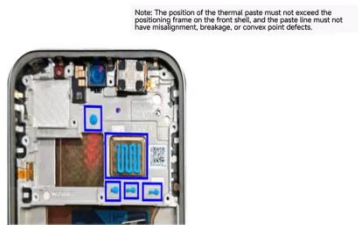
First, use a dispensing gun to apply thermal grease to the frame.
