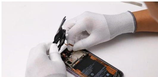
Fasten the flash FPC connector.
