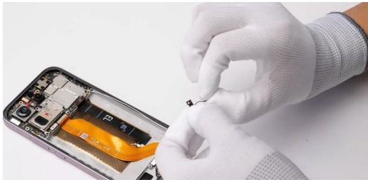
Couple the coaxial cable to the antenna board.
