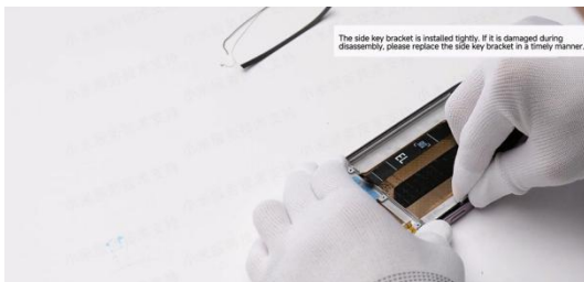
Use tweezers to lift the side key bracket from
