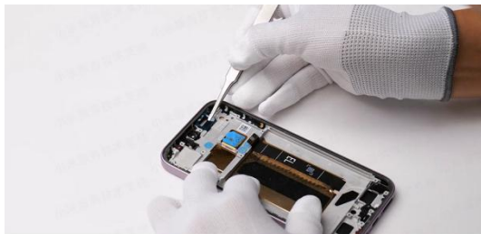
Apply the back glue to the receiver.
