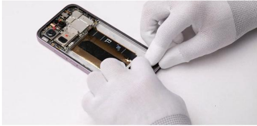
Make sure the sub-board is installed flat and without warping.
