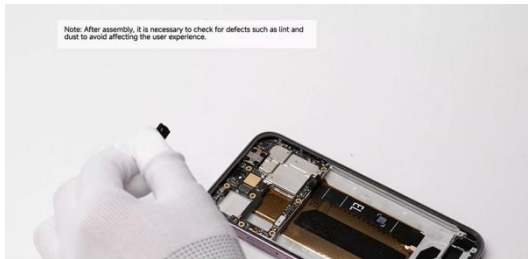
Remove the dust cover.
