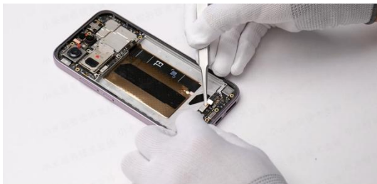
Install the fingerprint module and snap it to the sub-board.
