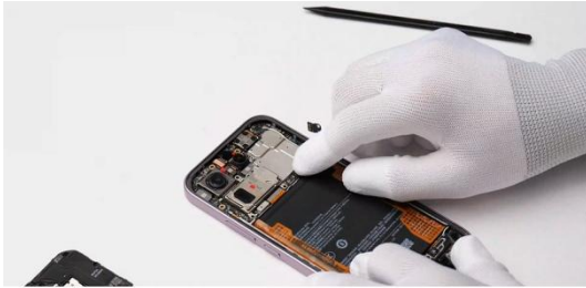
Use your fingertip to engage the screen FPC connector.
