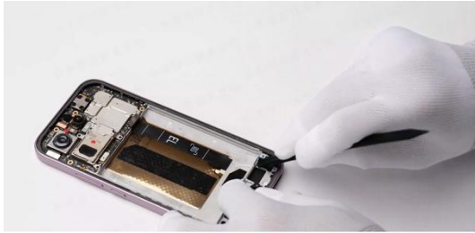
Tear off the release paper.
