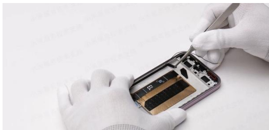
Tear off the coaxial cable from the middle frame.
