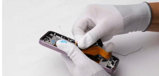
Check if the VC heat sink is wrinkle-free and deformed.
