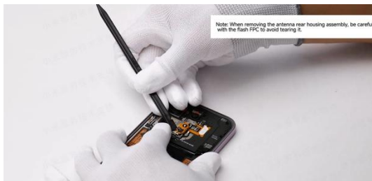
separate the flash FPC from the front camera.
