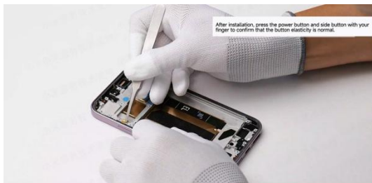
Then insert the side key FPC gold fingers
