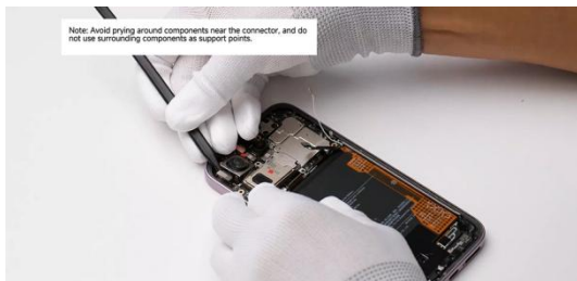
Use a pry bar to disconnect the rear main camera,
