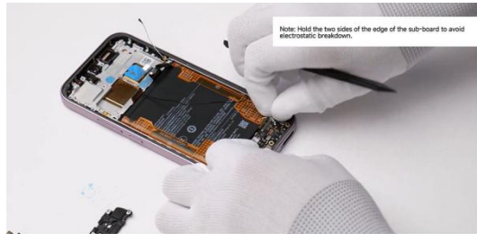
and gently lift and remove the sub-board.
