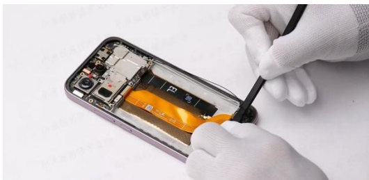
Then, insert the black and white coaxial cables into the slot.
