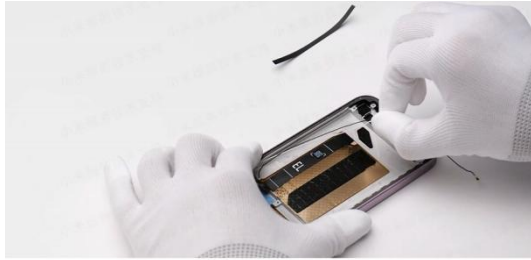
Remove the black and white coaxial cables.
