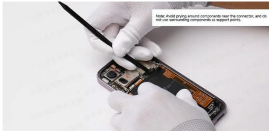
Disconnect the FPC connector.
