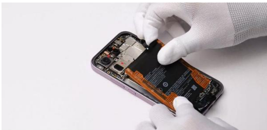
Assemble the battery into the middle frame battery compartment.
