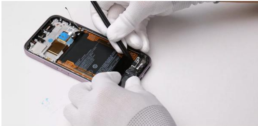
Remove the speaker assembly.
