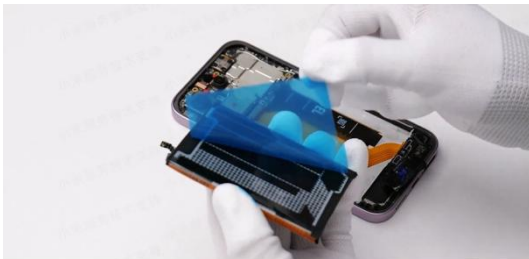
Peel off the battery's one-side adhesive release paper.
