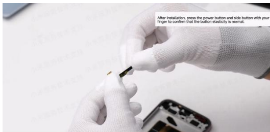
Insert the side key FPC assembly into the key slot of the side key bracket.
