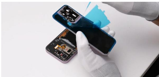
Peel off the back glue of the battery cover.
