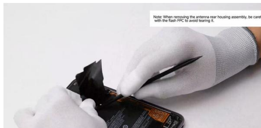
Lift it from the bottom of the antenna back shell.
