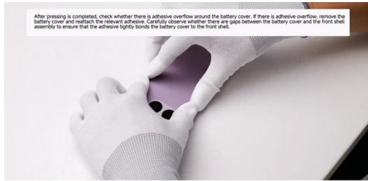
Insert the battery cover and press it.
