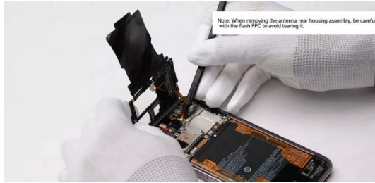
Disconnect the flash FPC BTB interface.
