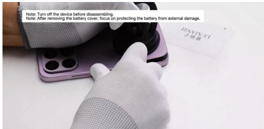
Remove the battery cover.
