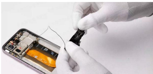
Insert the black coaxial cable into the speaker slot.
