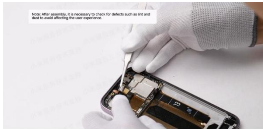
After confirming no defects, fasten the connector interface.
