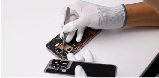
Remove the rear camera's protective film.
