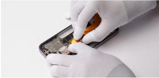
Fasten the main FPC interface of the main and sub boards.
