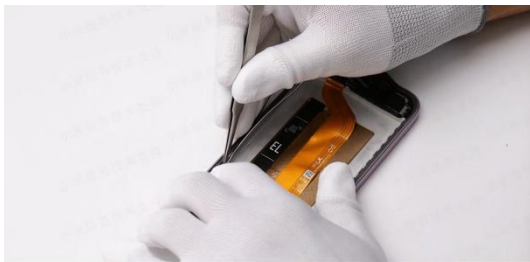
Fasten the black coaxial cable to the main board end.
