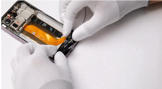
Assemble the lower speaker into the corresponding position.
