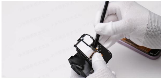
Disassemble the flash FPC component from the antenna back shell.
