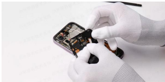
Assemble the flash FPC to the antenna back shell assembly.
