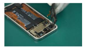
Pay attention to the clips around the Mainboard Cover Assy during operation. Make sure the clips are completely separated before proceeding to the next step to avoid damaging the Mainboard Cover Assy.
