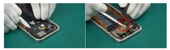
(3) Remove the Mainboard Cover Assy.
