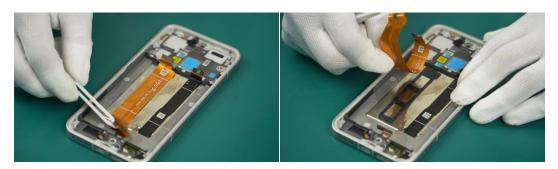
② You can use special alcohol to help remove the adhesive, or use the microwave to heat the heating bags, then heat the device before removing it.
