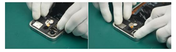
(3) Align the screw holes and tighten the screws.
