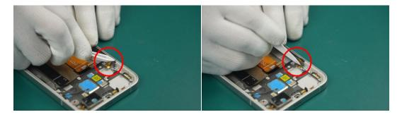
During the subsequent assembly process, you need to check whether the Holder-Side Key FPC cable is lifted up to avoid squeezing the cable during assembly.
