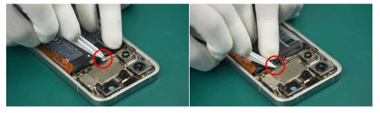
You can press the wiring harness interface with your fingers. If you can clearly feel a "click" sound, it means the interface is connected in place.
