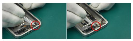
(2) After arranging the Coaxial Cables in the correct position, press the Mylar-Coaxial Cable tightly to ensure firm adhesion.
