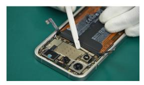
(3) Disconnect the Front Cover Display Module from the Mainboard Assy.
