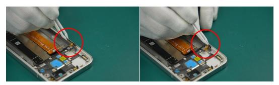
(2) then arrange the cable to ensure it is installed in place.
