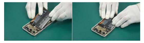
(3) Finally connect the Battery to the Mainboard Assy.
