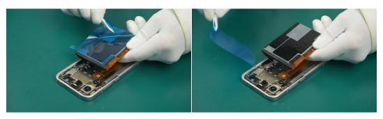
(2) Align the phone to the correct position, put the Battery in, and press lightly to ensure a firm fit.
