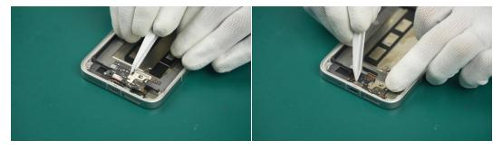
Please check the components underneath when installing the Sub-Board Assy. If the components underneath are not properly installed, the Sub-Board Assy may not be properly installed.
