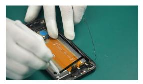
(2) Remove the Coaxial Cable-White from the device.
