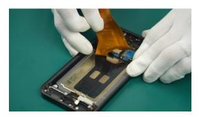
② You can use special alcohol to help remove the adhesive, or use the microwave to heat the heating bags, then heat the device before removing it.
