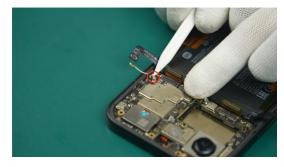
Do not pull the cable directly when disconnecting to avoid breaking it.
