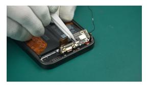
Pay attention to the clips around the Sub-Board Assy during operation. Make sure the clips are completely separated before proceeding to the next step to avoid damaging the Sub-Board Assy.
