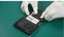
(4) Tear off the protective film on the other side of the Battery Cover Adhesive.
