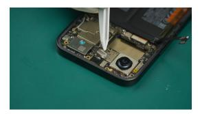
When peeling off the radiation Copper Foil, handle it carefully to avoid tearing it forcefully and causing damage.
