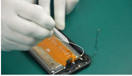
• Be careful not to damage the wiring harness interface and surrounding components during operation.
