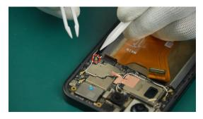
You can press the wiring harness interface with your fingers. If you can clearly feel a "click" sound, it means the interface is connected in place. (3) Connect the Main FPC Assy to the Mainboard Assy.
