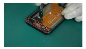
Please make sure that all the clips are in place, otherwise it will affect the subsequent assembly. Check the number of screws installed to ensure that no unassembled screws are left inside the device during the assembly process.
