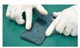
(3) Tear off the protective film on the other side of the Adhesive-Battery Cover, install the Battery Cover, and press to ensure a firm fit.
