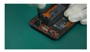
(2) Use tweezers to separate the Antenna Board Assy and Coaxial Cable-Black from the Speaker Assy.
