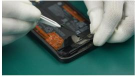
(3) Remove the Speaker Assy from the device.
