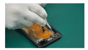
(5) Tighten the screws of the Sub-Board Assy one by one.
