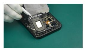
Pay attention to the clips around the Holder Assy during operation. Make sure the clips are completely separated before proceeding to the next step to avoid damaging the Holder Assy.
