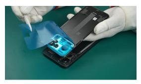
(5) Align the Battery Cover Assy with the device, and press gently to install it in place.
