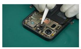
(2) Disconnect Camera-Rear-Ultra-Wide Angle and remove it from the device.
