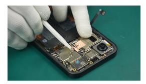
(6) Disconnect and remove the Coaxial Cable-White.
