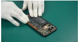
(3) Connect the Battery to the Mainboard Assy.
