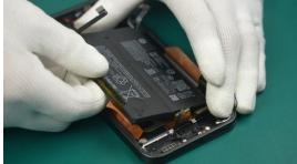
(2) Tear off the remaining Easy Release Adhesive on the device.
