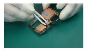
(4) Place the Mainboard Assy into the device and press firmly into place.
