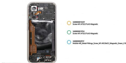
Use a screwdriver to install all screws
