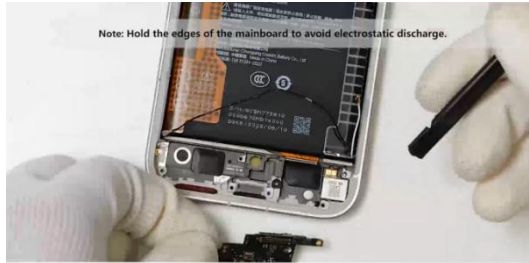
Use a prying tool to gently pry up and remove the sub-board from the sub-board disassembly position
