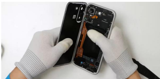
After disassembling, clean the residual glue on the battery cover plate and the middle frame until the residual glue is completely removed
