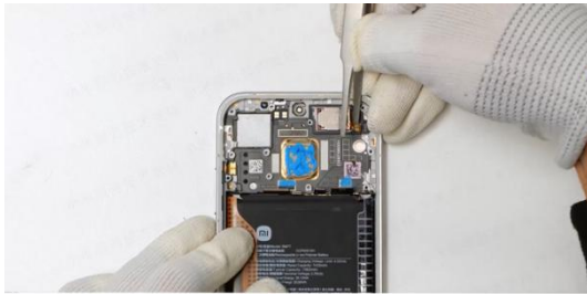
Use tweezers to pry up the earpiece FPC from the earpiece FPC disassembly position
