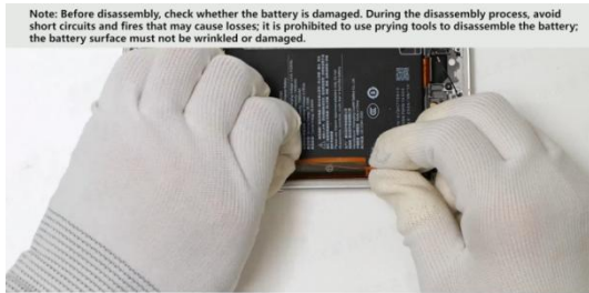
Peel off the yellow and transparent adhesive tapes on the battery
