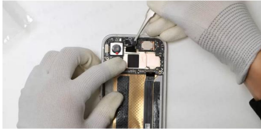
Apply new conductive fabric to the front camera area and press it
