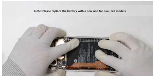
Note: Please replace the battery with a new one for dual-cell models Use a fixture to attach the new battery spare part to the battery, peel off the release paper privately, and install the battery in place
