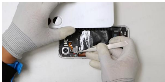
Remove the protective film from the camera
