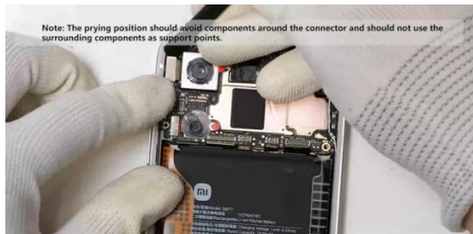
Use a pry tool to disconnect the connectors of the rear main camera lens and the wide-angle lens, and then remove them.
