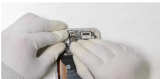
Gently pry up and remove the light sensor board
