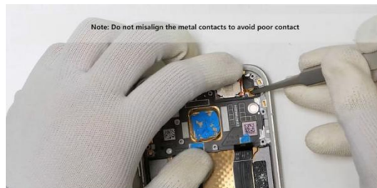
Arrange and paste the earpiece FPC into the limit slot of the middle frame, ensuring it is flat and without warping
