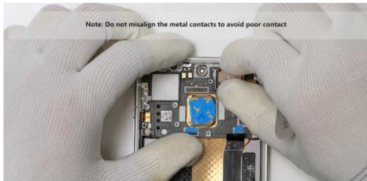
Install the earpiece, gently press it to activate the adhesive backing
