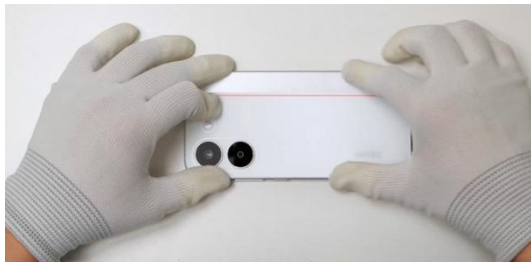
Then press and secure the entire battery cover in place, and press down on all four edges of the battery cover by hand to ensure it is properly installed and aligned
