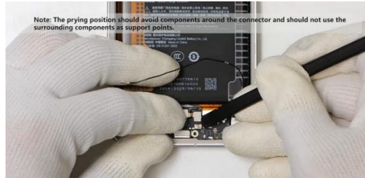
Disconnect the coaxial connector, fingerprint connector, and main FPC connector
