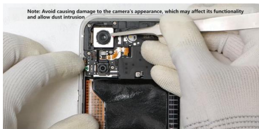
Use a camera cover or protective film to protect the lens from dust and wear
