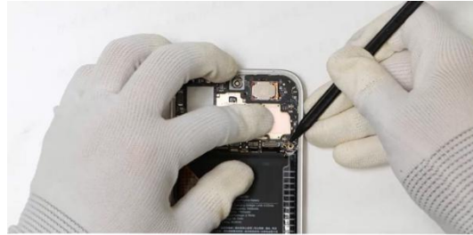
Disconnect the black and white axes of the mainboard
