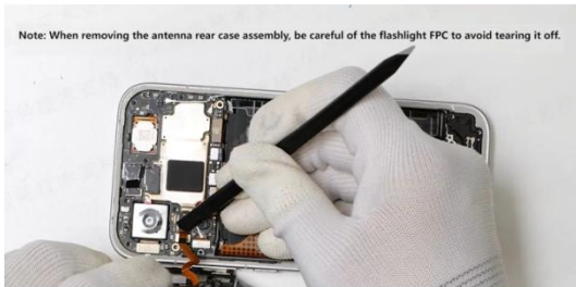
Disconnect the flashlight FPC interface
