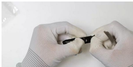
Connect the coaxial cable to the antenna sub-board, route the coaxial cable into the cable slot, and then assemble it to the corresponding position of the lower speaker
