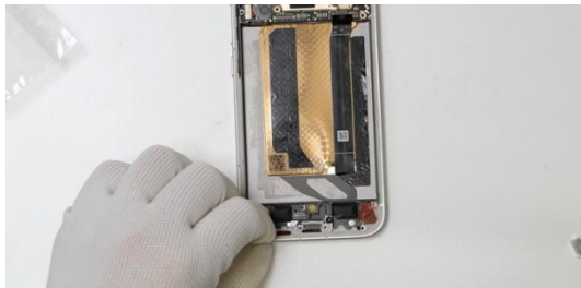
Paste the motor adhesive backing and remove the release paper
