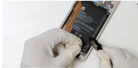
Separate the antenna sub-board from the lower speaker and disconnect the coaxial cable from the sub-board
