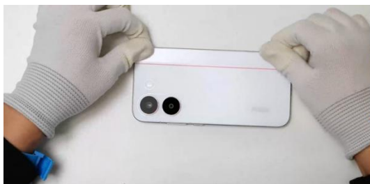
Place it into the battery cover pressing fixture to secure
