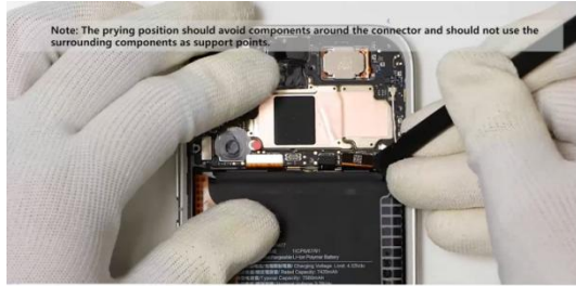
Disconnect the display FPC connector and the main FPC connector
