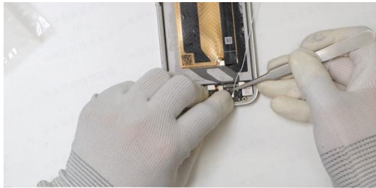
The white coaxial cable is snapped into the connection base of the sub-board
