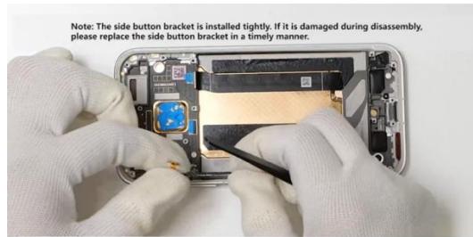
Use tweezers to pry up and remove the side button bracket from the middle frame
