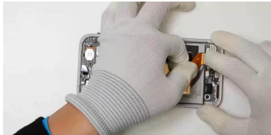
The main FPC connector is respectively fastened to the sub-board and the main board, and then pasted securely
