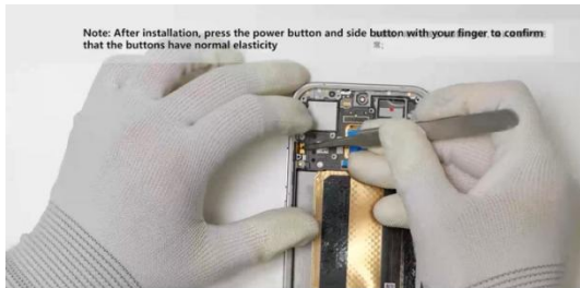
Install the FPC gold finger of the side button into the corresponding position of the middle frame
