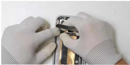
Engage the connector interface, ensuring it is fully engaged, flat, and without any lifting
