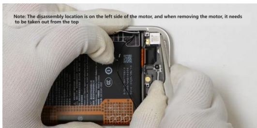
Use tweezers to pry up the motor from the disassembly position on the side of the motor and remove it
