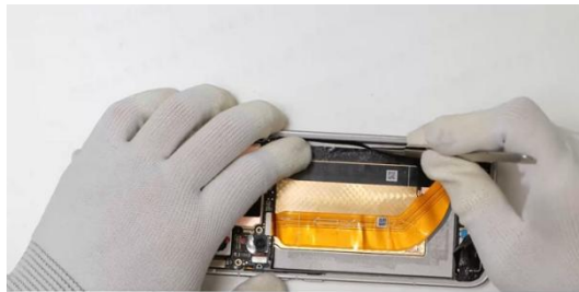
Insert into the middle frame slot and add the middle frame coaxial cable mylar
