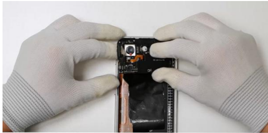
Snap the flashlight FPC connector into place, and then snap the antenna rear case assembly onto the middle frame along the top of the middle frame
