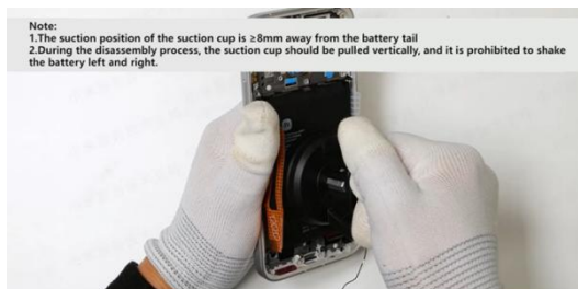
Use a suction cup to slowly and uniformly pull the battery vertically upward
