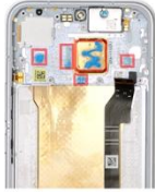
First, use a dispenser to apply thermal paste on the middle frame
