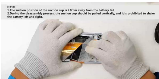
After disassembly, check the appearance of the battery. If there is any damage or deformation, replace it promptly.
