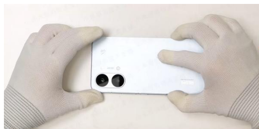
Align one end of the battery cover (with adhesive applied) with the front case assembly
