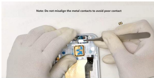
Paste the back adhesive of the earpiece and remove the release paper
