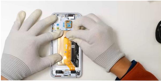
Slowly peel off the main FPC, and check if the VC heat sink has any wrinkles or deformations
