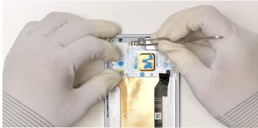
Install the light sensor board into the front case subassembly
