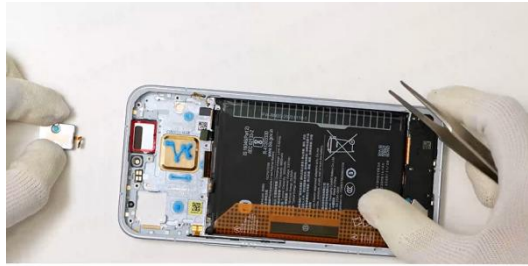
Use tweezers to pry up and remove the earpiece at the disassembly position on the left side of the earpiece; remove the double-sided adhesive tape for earpiece sealing
