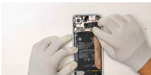
Snap in the BTB cable, and confirm that the cable is not lifted (first snap in battery BTB1, then snap in BTB2)
