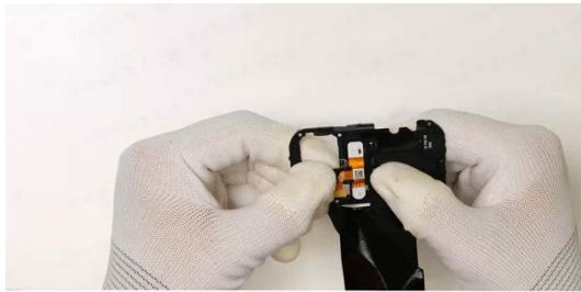
Install the flashlight FPC onto the antenna rear case assembly
