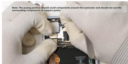
Remove the graphite copper foil of the front camera
