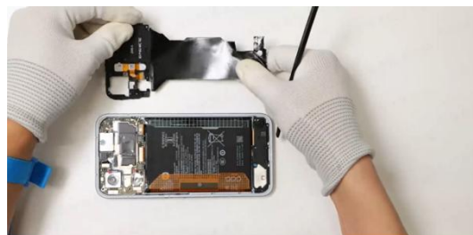
Lift the graphite sheet, remove the antenna rear case assembly by lifting it from the bottom of the antenna rear case assembly
