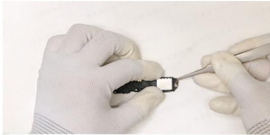
Install the lower speaker assembly along the lower edge of the middle frame without warping or tilting
