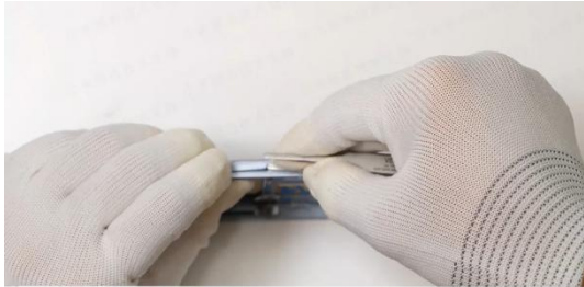
Use tweezers to push out the power button and volume button, then remove them
