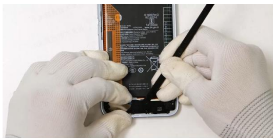
Use your hand or a prying tool at the disassembly position above the speaker to remove the speaker assembly
