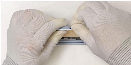
Install the volume button and power button into the button slots on the middle frame
