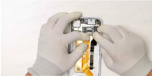
Snap the mainboard display FPC interface
