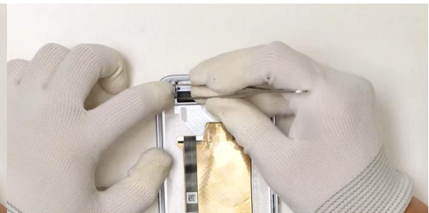
Use tweezers to pick up the vibrator, vertically assemble it into the limit slot of the middle frame, and gently press to activate the adhesive
