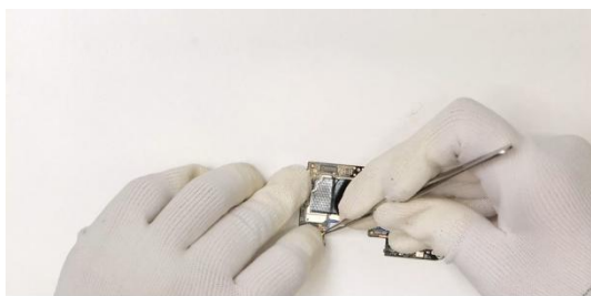
Install the blue coaxial cable on the mainboard
