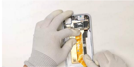
Snap the mainboard display FPC interface
