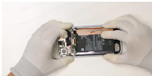
Use a fixture to attach the new battery spare part to the battery, peel off the release paper privately, and install the battery in place
