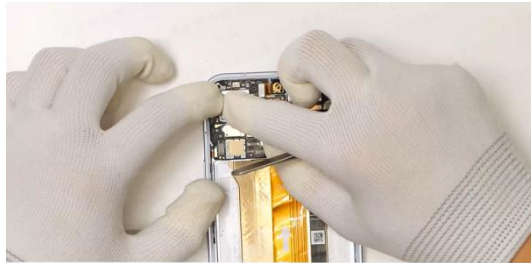
Install the rear main camera and wide-angle camera to the corresponding positions on the mainboard
