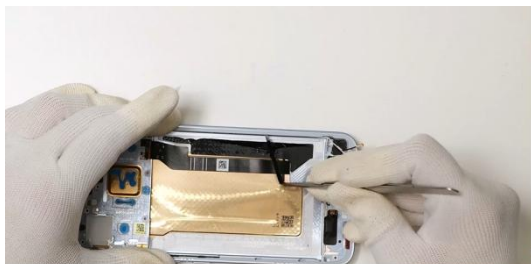
Remove the middle frame coaxial cable Mylar, and take out the black and white coaxial cables
