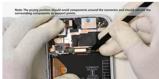
Use anti-static plastic tweezers or pry tools to sequentially disconnect the #2 and #1 battery connectors
