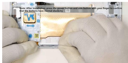
Combine the side button FPC with the bracket and install it into the middle frame
