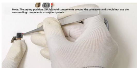
Use a pry tool to disconnect the front camera FPC connector and remove it, then protect the camera
