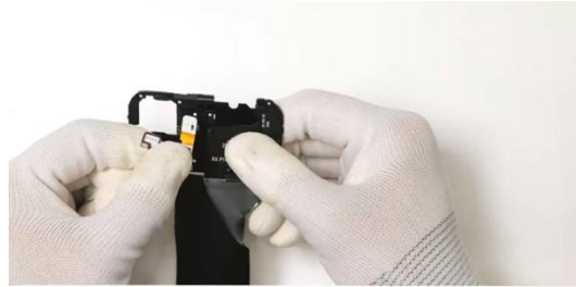
Separate the flashlight FPC assembly from the antenna rear case assembly
