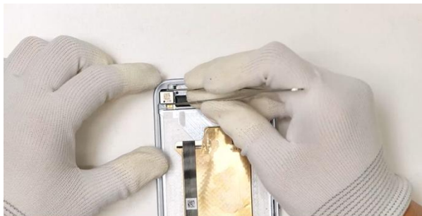
Use tweezers to pick up the vibrator, vertically assemble it into the limit slot of the middle frame, and gently press to activate the adhesive
