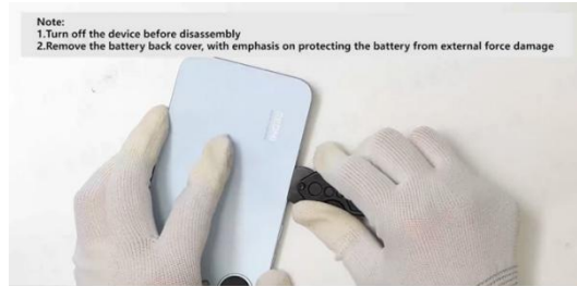
After heating, use the suction cup to lift the gap and insert the disassembly blade into the gap along the side or bottom of the battery cover
