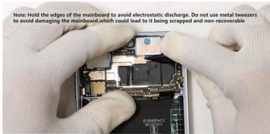
Remove the earpiece grounding copper foil
