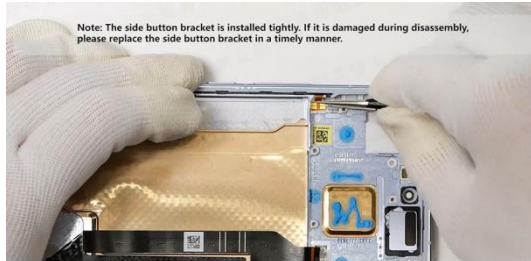
Gently pry up the side button FPC gold finger from the disassembly position
