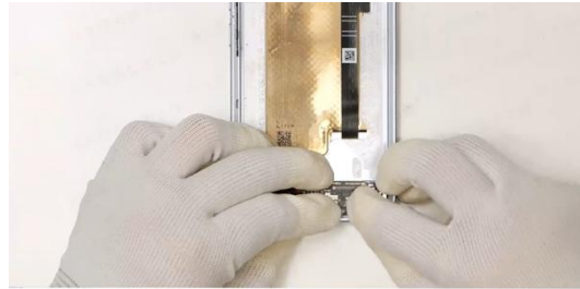
Along the lower edge of the middle frame, tilt and assemble the sub-board onto the middle frame, ensuring that the sub-board is installed flat and without warping
