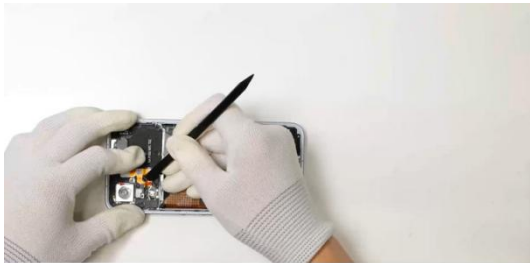
Disconnect the flashlight FPC interface
