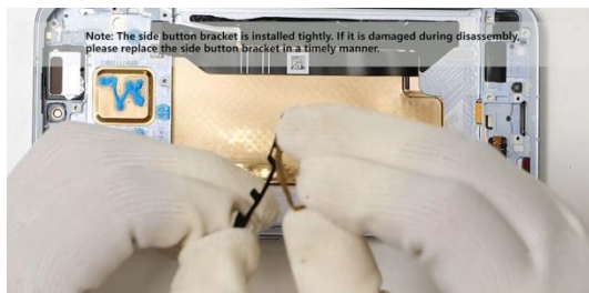
Separate the side button FPC from the side button bracket
