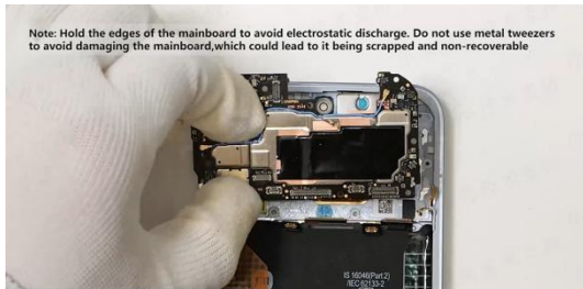
Remove the mainboard at the notch position of the main camera on the mainboard
