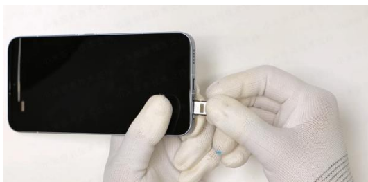
Ensure the correct orientation of the SIM card tray, Insert vertically into the phone's SIM card tray
