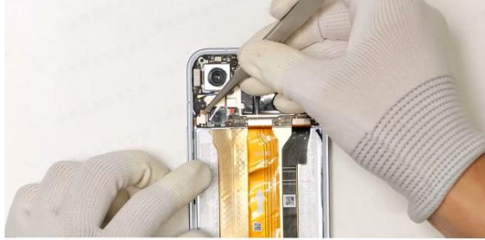
Sequentially attach the earpiece grounding copper foil, front camera graphite copper foil, and wide-angle camera BTB grounding copper foil
