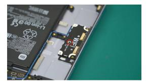
(2) Use tweezers to remove the Wi-Fi module.
