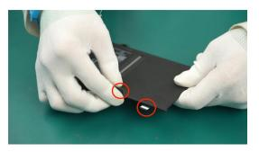
(3) Remove the sticker of the Easy Pull Tape and put the Battery in the correct position of the tablet.
