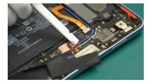
(2) Use the plastic pry bar to open the other buckle of the Coaxial Cable-White.
