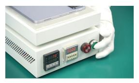
(2) Place the tablet on the heating platform and continue heating for 1-2 minutes.
