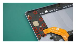
(2) Place the Top right speaker in the correct position and tighten the speaker screws.
