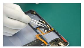
(2) Tighten the Wi-Fi Module screw.
