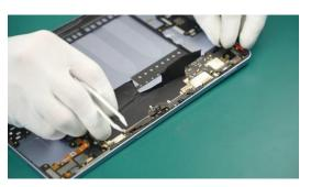
Do not touch the Mainboard Assy directly with metal tools to avoid scratching the Mainboard Assy and static damage.
