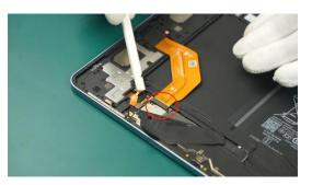
(2) Disconnect the FPC-POGOPIN cable from the Mainboard Assy.
