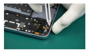
(2) Use tweezers to install the Limit Sheet Steel into the correct position.
