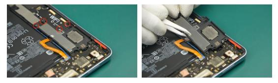
(2) Use a phillips screwdriver to remove the screws on the Speaker Assy (Lower left).
