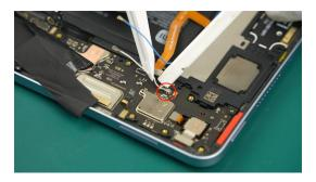
(3) Use tweezers to remove the Coaxial Cable-White.
