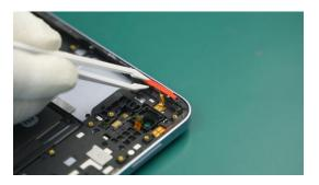
(2) Remove the Limit Sheet Steel using tweezers.
