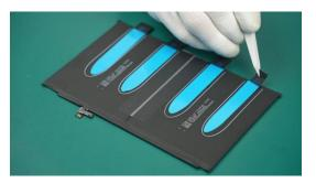
Before attaching the new Easy Pull Tape, please clean the remaining Easy Pull Tape.
