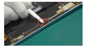
You can press the wiring harness interface with your fingers. If you can clearly feel a "click" sound, it means the interface is connected in place.
