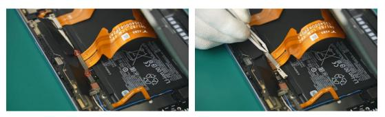
Check the number of screws that have been removed and keep them in a safe place to ensure that no unassembled screws are left inside the device during the assembly process.
