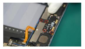
Check the number of screws installed to ensure that no unassembled screws were left inside the device during assembly.
