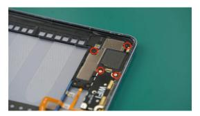
(2) Place the Top left speaker in the correct position and tighten the speaker screws.
