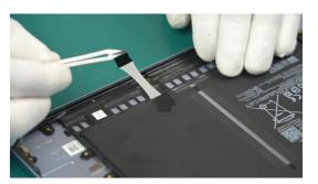
(2) Use the Plastic Pry Bar to pry up the Battery and remove it.
