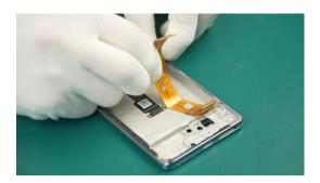
② You can use special alcohol to help remove the adhesive, or use the microwave to heat the heating bags, then heat the device by the heating bags before removing it.
