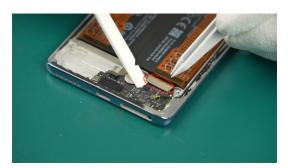
(3) Disconnect and remove the Coaxial Cable.
