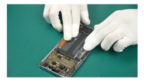
(3) Connect the Battery to the Mainboard Assy.
