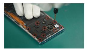
Please check the number of screws installed to ensure that no unassembled screws are left inside the device.
