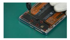
Check the number of screws that have been removed and keep them in a safe place to ensure that no unassembled Screws are left inside the device during the assembly process.
