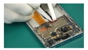
You can press the wiring harness interface with your fingers. If you can clearly feel a "click" sound, it means the interface is connected in place.
