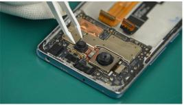
• Do not touch the camera lens directly during operation to avoid scratching the lens.
