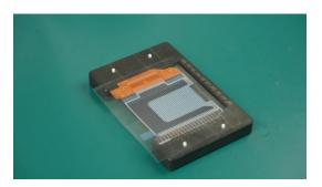
(2) Tear off the protective film, try to avoid touching the adhesive surface to prevent it from being contaminated and affecting the assembly effect, then align and attach the Battery.
