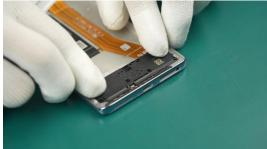
During assembly, carefully check the lower harness to ensure that it is installed in the wire guide and do not allow the Speaker Assy to squeeze the lower harness.
