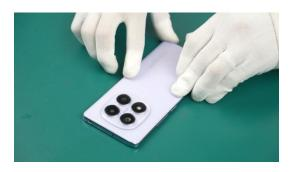
Place the phone into the Battery cover assembly press device and press for 60 seconds using the Crimping tool.
