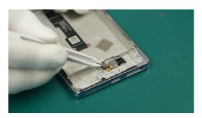
Check whether the Fingerprint module is installed properly. If the Fingerprint module is not installed properly, it may affect subsequent installations.
