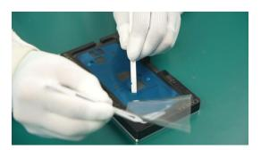
(3) Put the Battery Cover Assy into the Adhesive backing fixing tool, press gently to make the Battery Cover Adhesive and the Battery Cover Assy fit together.
