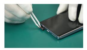
Please do not use hard tools to install the SIM card tray to avoid scratching the device.
