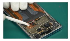
(3) Disconnect the FPC Assy-TP Transfer from the Mainboard Assy.
