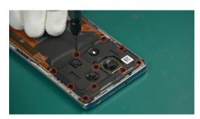
Check the number of screws that have been removed and keep them in a safe place to ensure that no unassembled screws are left inside the device during the assembly process.
