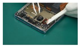
Do not touch the camera lens directly during operation to avoid scratching the lens.
