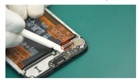
Please disconnect the interface in parallel during operation to avoid tilting and pulling, which may cause damage to the interface.
