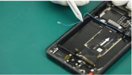
Please carefully tear off the Coaxial Cable Tray Blocking Foam. Do not use brute force, as this may damage the Coaxial Cable Tray Blocking Foam.
