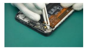
Please tear the Conductive Cloth-Vibrator carefully without damaging it. If the Conductive Cloth-Vibrator is too tightly bonded, you can use special alcohol to assist the operation. (5) Remove the Sub-Board Assy.
