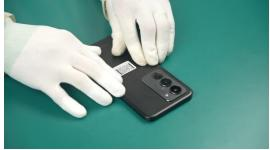
Before attaching the new Adhesive-Battery Cover, please clean the remaining Adhesive-Battery Cover.
