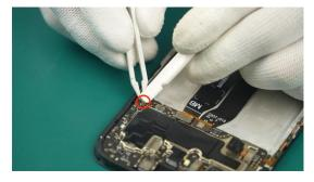
② You can press the wiring harness interface with your fingers. If you can clearly feel a "click" sound, it means the interface is connected in place.
