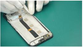
Please ensure that the Coaxial Cable Tray Blocking Foam fits flatly, otherwise it will affect subsequent installation.
