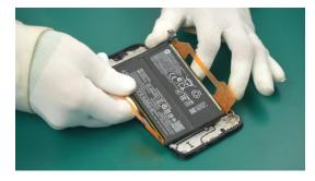
(3) Remove any remaining Easy Release Adhesive from the device.
