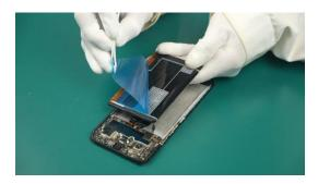
(6) Align the phone to the correct position, put the Battery in, and press lightly to ensure a firm fit.
