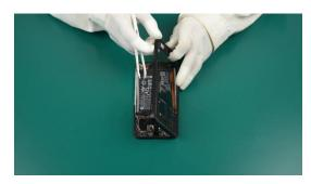
(3) Connect the cable of the Fingerprint Module to the Mainboard Assy.
