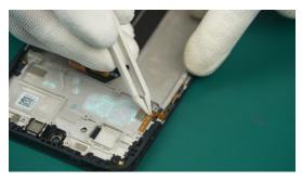
During the subsequent assembly process, you need to check whether the FPC Assy-Side Key is lifted up to avoid squeezing the harness during assembly.
