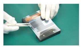
(2) Tear off the protective film of the Easy Release Adhesive, and try to avoid touching the adhesive surface to prevent it from being contaminated and affecting the installation effect.
