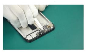
(2) Press the Sub-Board Assy gently to ensure it is properly installed.
