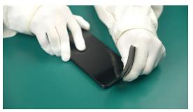
You can use a Plastic Pry Bar to pry open the fixing clips. Please be careful not to use brute force to avoid damaging the device. (4) Lift the Middle Frame Assy and disconnect the cable of the Fingerprint Module from the device, then remove the Middle Frame Assy.
