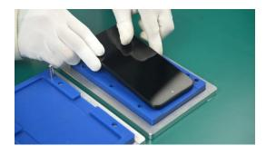
(2) Press for 60 seconds using the Crimping tool.
