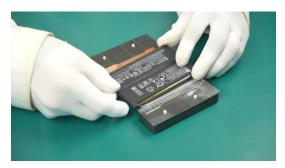
(4) Tear off the protective film on the other side of the Easy Release Adhesive.
