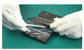
(5) Tear off the protective film on the back of the Easy Release Adhesive.
