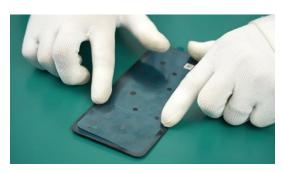
(4) Tear off the protective film on the other side of the Adhesive-Battery Cover, install the Battery Cover, and press to ensure a firm fit.
