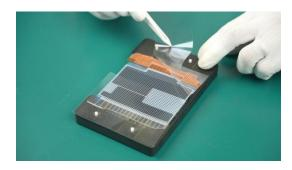
(3) Align and attach the Battery.
