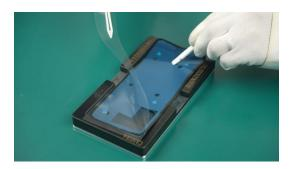
(3) Put the Battery Cover Assy into the Adhesive backing fixing tool, and press gently to make the Battery Cover Adhesive and the Battery Cover Assy fit together.
