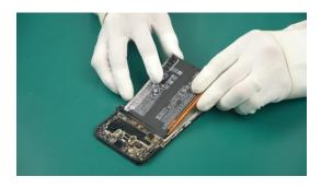
(7) Connect the Battery to the Mainboard Assy.
