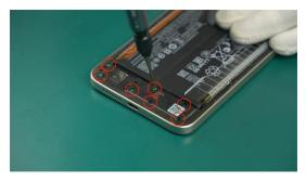
Please check the number of screws installed to ensure that no unassembled screws are left inside the device.
