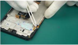
(2) Tidy up the wire harness to ensure it is installed in place.
