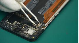
(3) Disconnect Camera-Front and remove it from the device.
