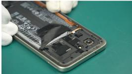
(4) Tighten the Middle Frame Assy screws one by one.
