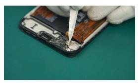
(5) Remove the Sub-Board Assy from the device.
