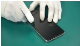
(3) Lift the Middle Frame Assy. Disconnect the cable of the Fingerprint Module from the device, and then remove the Middle Frame Assy;
