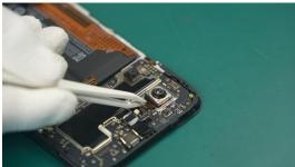
(2) Disconnect Camera-Rear-Macro-Depth and remove it from the device.
