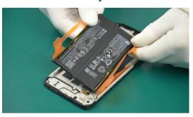
(2) Tear off the remaining Easy Release Adhesive on the device.
