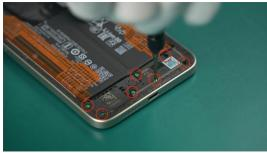
Check the number of screws that have been removed and keep them in a safe place to ensure that no unassembled screws are left inside the device during the assembly
