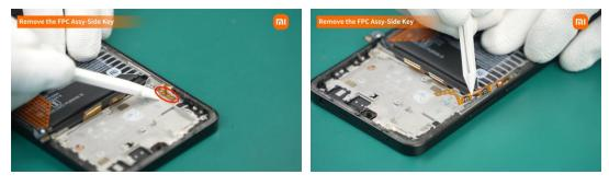
Carefully disconnect the adhesive and remove the FPC Assy-Side Key.
