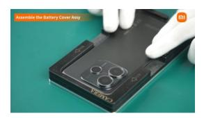
(4) Tear off the protective film on the other side of the Battery Cover Adhesive, align the Battery Cover Assy with the device, and press gently to install it in place.
