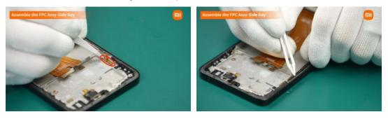
During the subsequent assembly process, you need to check whether the Holder-Side Key FPC harness is lifted up to avoid squeezing the harness during assembly.
