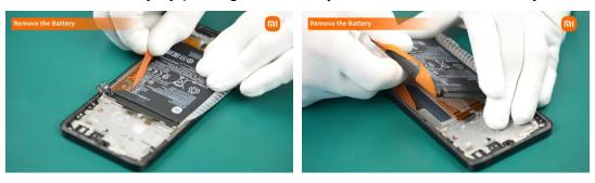
(2) Tear off the remaining Easy Release Adhesive-Battery on the device.
