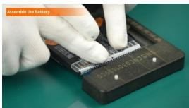
(4) Then tear off the protective film on the back of the Easy Release Adhesive, align the phone to the correct position, then put the Battery in.
