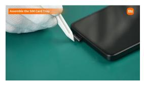
Please do not use hard tools to install the SIM card tray to avoid scratching the device.
