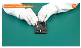
Pay attention to the clips around the Flash Light Board Assy during operation. Make sure the clips are completely separated before proceeding to the next step to avoid damaging the Flash Light Board Assy.
