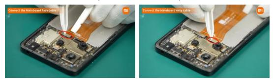
② You can press the wiring harness interface with your fingers. If you can clearly feel a "click" sound, it means the interface is connected in place.
