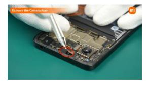
Please be careful to avoid damaging the Conductive Copper Foil.
