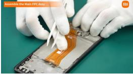
Please ensure that the Main FPC Assy fits flatly with the device to avoid damage to the Main FPC Assy caused by squeezing other accessories during subsequent assembly.
