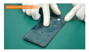
(3) Tear off the protective film on the other side of the Adhesive-Battery Cover, install the Battery Cover, and press to ensure a firm fit.
