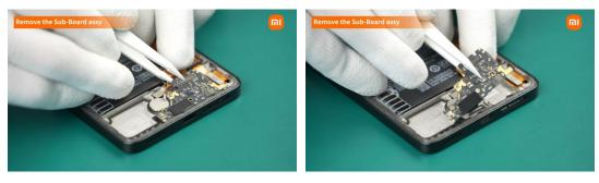
Pay attention to the clips around the Sub-Board Assy during operation. Make sure the clips are completely separated before proceeding to the next step to avoid damaging the Sub-Board Assy.
