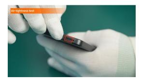
(2) Use the Air tightness tester, aim at the air tightness test hole, and perform the test. If "OK" is displayed on the screen, it means that the mobile phone has passed the test.
