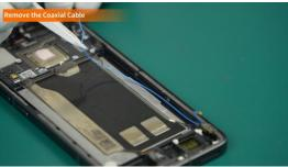
Do not pull the interface of the Coaxial Cable to avoid breaking the interface of the Coaxial Cable.
