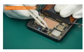
(5) Disconnect the Camera-Front and remove it from the device.
