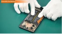
(7) Connect the Battery to the Mainboard Assy.
