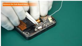
Pay attention to the clips around the Sub-Board Assy during operation. Make sure the clips are completely separated before proceeding to the next step to avoid damaging the Sub-Board Assy.
