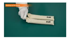
🔼 Use the label as a handle when removing the Heating Bag to avoid burns.
