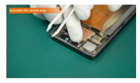
Attach the Copper Foil flatly. You can press lightly with your fingers to ensure it fits securely. (3) Place the Camera-Rear-Main in the correct position of the device and connect it to the Mainboard Assy.
