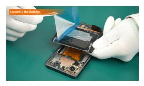
(6) Align the phone to the correct position, put the Battery in, and press lightly to ensure a firm fit.
