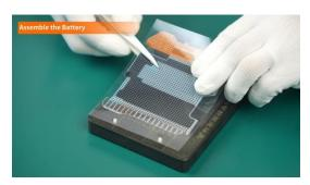
(2) Tear off the protective film of the Easy Release Adhesive, and try to avoid touching the adhesive surface to prevent it from being contaminated and affecting the installation effect.
