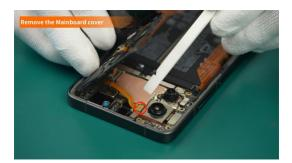
Pay attention to the clips around the Mainboard Cover Assy during operation. Make sure the clips are completely separated before proceeding to the next step to avoid damaging the Mainboard Cover Assy.
