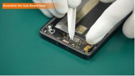
Please check the components underneath when installing the Sub-Board Assy. If the components underneath are not properly installed, the Sub-Board Assy may not be properly installed.
