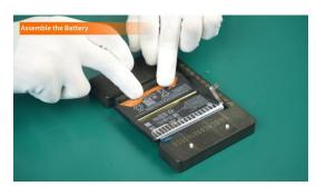
(5) Tear off the protective film on the back of the Easy Release Adhesive.
