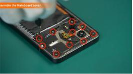
Please check the number of screws installed to ensure that no unassembled screws are left inside the device.
