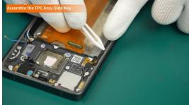
② You can press the wiring harness interface with your fingers. If you can clearly feel a "click" sound, it means the interface is connected in place.
