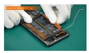
(2) Remove the Battery and tear off the remaining Easy Release Adhesive on the device.
