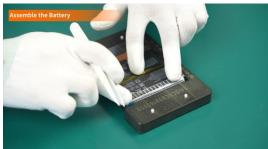
(4) Tear off the protective film on the other side of the Easy Release Adhesive.
