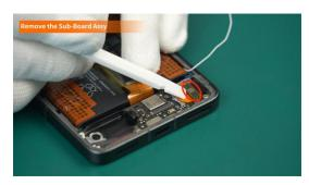
(7) Disconnect the Coaxial Cable-Blue from the Sub-Board Assy.
