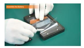
(3) Align and attach the battery.
