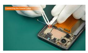
(2) Connect the Coaxial Cable-Blue to the Mainboard Assy and organize the cables.
