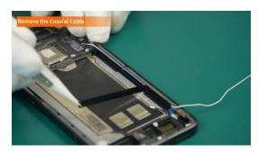
(2) Remove the Coaxial Cable-White and Coaxial Cable-Blue from the device.
