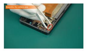
(5) Install the Camera-Rear-Ultra Wide Angle and connect it to the Mainboard Assy.
