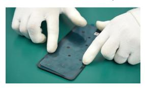
(4) Tear off the protective film on the other side of the Battery Cover Adhesive, install the Battery Cover Assy, and press to ensure a firm fit.
