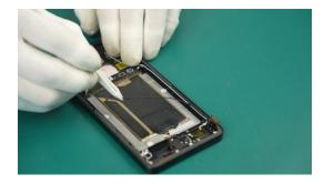
(2) Remove the Coaxial Cable-White from the cable trough.
