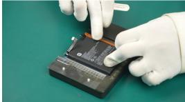
(3) Tear off the protective film on the other side of the Easy Release Adhesive, and try to avoid touching the adhesive surface.
