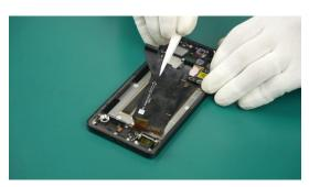
You can use special alcohol to help remove the adhesive, or use the microwave to heat the heating bags, then heat the device before removing it.
