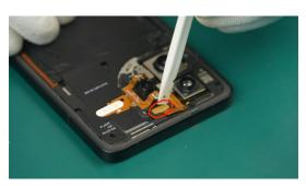
(2) Use a needle screwdriver to remove the screws.
