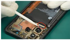
Please disconnect the interface in parallel during operation to avoid tilting and pulling, which may cause damage to the interface.
