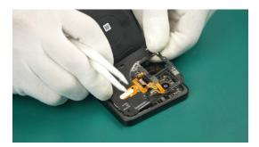
You can use a Plastic Pry Bar to open the fixing clips. Please be careful not to use brute force to avoid damaging the device.
