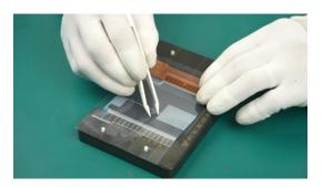
(2) Tear off the protective film, try to avoid touching the adhesive surface to prevent it from being contaminated and affecting the assembly effect, then align and attach the batteries.
