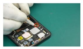
During the subsequent installation process, you need to check whether the Side Key FPC harness is lifted up to avoid squeezing the harness during installation.
