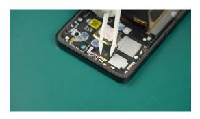
Do not use metal tools to press to avoid damaging the Light Sensor Board Assy.
