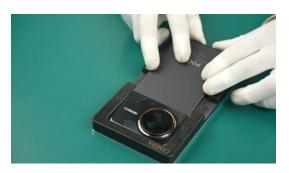
(5) Tear off the protective film on the other side of the Battery Cover Adhesive, align the Battery Cover Assy with the device, and press gently to install it in place.
