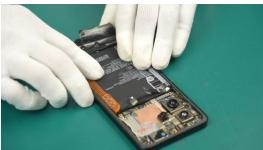
(5) Connect the Battery to the Mainboard Assy.
