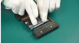
(4) Then tear off the protective film on the back of the Easy Release Adhesive, align the phone to the correct position, then put the Battery in.
