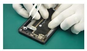
During the subsequent assembly process, you need to check whether the FPC Assy is lifted up to avoid squeezing the harness during assembly.
