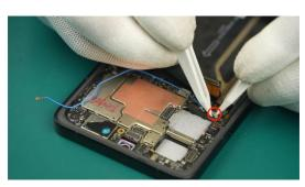
(2) Arrange the Coaxial Cable-Blue to the cable trough and connect the other end of the Coaxial Cable-Blue to the Mainboard Assy.
